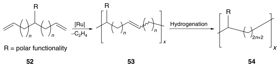
Figure 8.24 Using ADMET/hydrogenation to produce polyethylene with polar functionalities.
