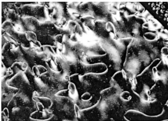
Fig. 5.3 Nematic liquid crystals of polymetallayne 5.2 ( M = \text{Pt} , L = \text{P}^n\text{Bu}_3 , x = 2 , n \approx 100 ) observed between cross-polarizers in trichloroethene at 25 °C. (We thank Prof. S. Takahashi, Osaka University, for the figure)
