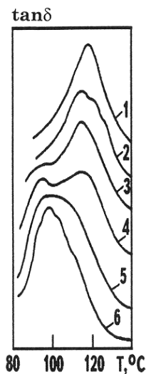
Figure 5.6. Transformation of curve \tan\delta=f(T) with variation of the ratio polymer/interphase 1-0.6, 2-0.7, 3-0.8, 4-0.9, 5-0.95, 6-0.99 for T_g=398\text{K} and T_m=373\text{K} .
