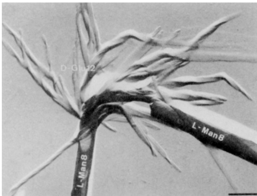
Figure 5.4 Electron micrograph showing demixing of D-Glu-12 helices from L-Man-8 tubules to form heterogeneous structures (bar = 500 nm). Reprinted with permission from Ref. 31. Copyright 1990 by the American Chemical Society.
