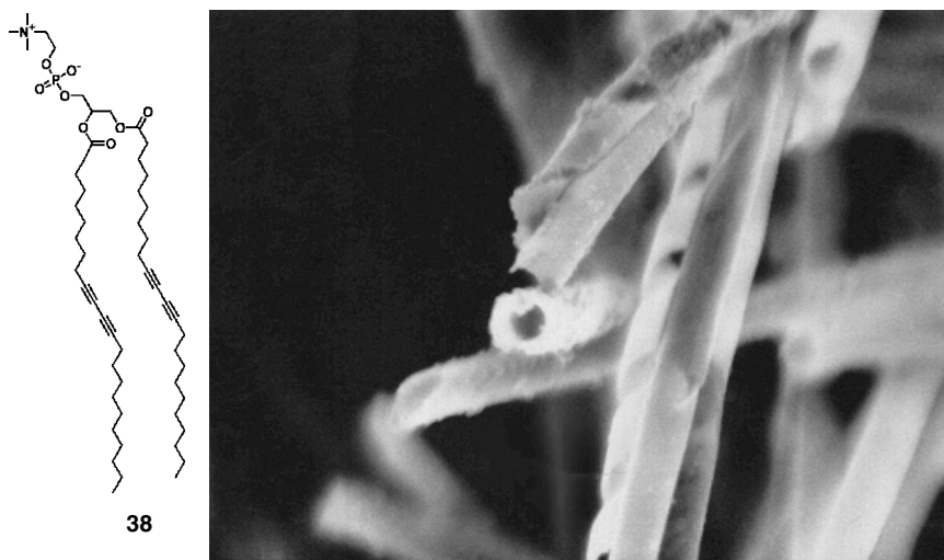
Figure 5.27 Scanning electron micrograph of copper-coated DC 8,9 PC ( 38 ) tubules. Tubules are hollow with diameter of approximately 0.5 \mu\text{m} (bar = 0.5 \mu\text{m} ). Helical wrappings evident in some tubules are all right handed. Reprinted with permission from Ref. 125. Copyright 1998 by the American Chemical Society.
