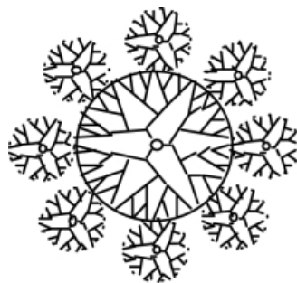
Figure 12.20 Schematic representation of a core-shell tecto-(dendrimer) molecule in solution
