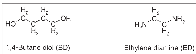
Fig. 1.6. Chain extenders commonly used for the synthesis of biomedical-grade polyurethanes.
