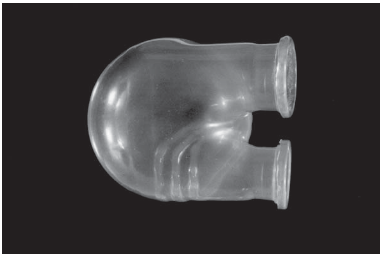
Fig. 8.10. Ventricle of ventricular assist device made of polyurethane: despite weaknesses in blood compatibility, it presents excellent flexure and wear properties.
