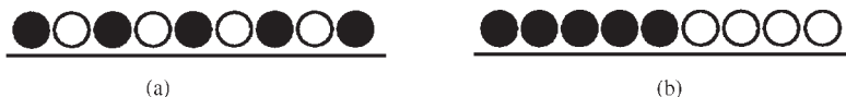
FIGURE 19. Possible arrangement in mixed monolayers: homogeneous mixture (a) or phase-separated domains (b)
