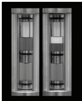
Figure 4. Left side: Miscible Solution of THF/water at 1 bar. Right side: phase separation at 30 bar CO 2 . The partition coefficient of the water-soluble dye is greater than 10 6 ! (14)
