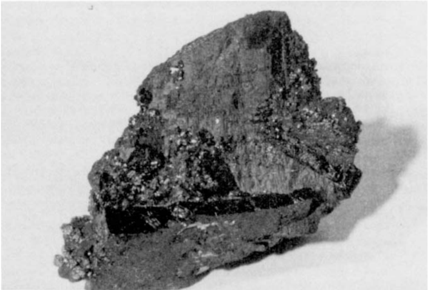
FIGURE 2.3. Huebnerite, Ferberite, and Scheelite: (a) Huebnerite : ruby red, transparent euhedral crystals; length about 6 cm; small white tetragonal scheelite crystals grown on top of them; Pasto Bueno Mine, Ancash, Peru. (b) Ferberite : black, plate-like crystals; dimensions 3 \times 5 cm; together with pyrite and arsenophrite; Palca XI Mine, Puno, Peru.
