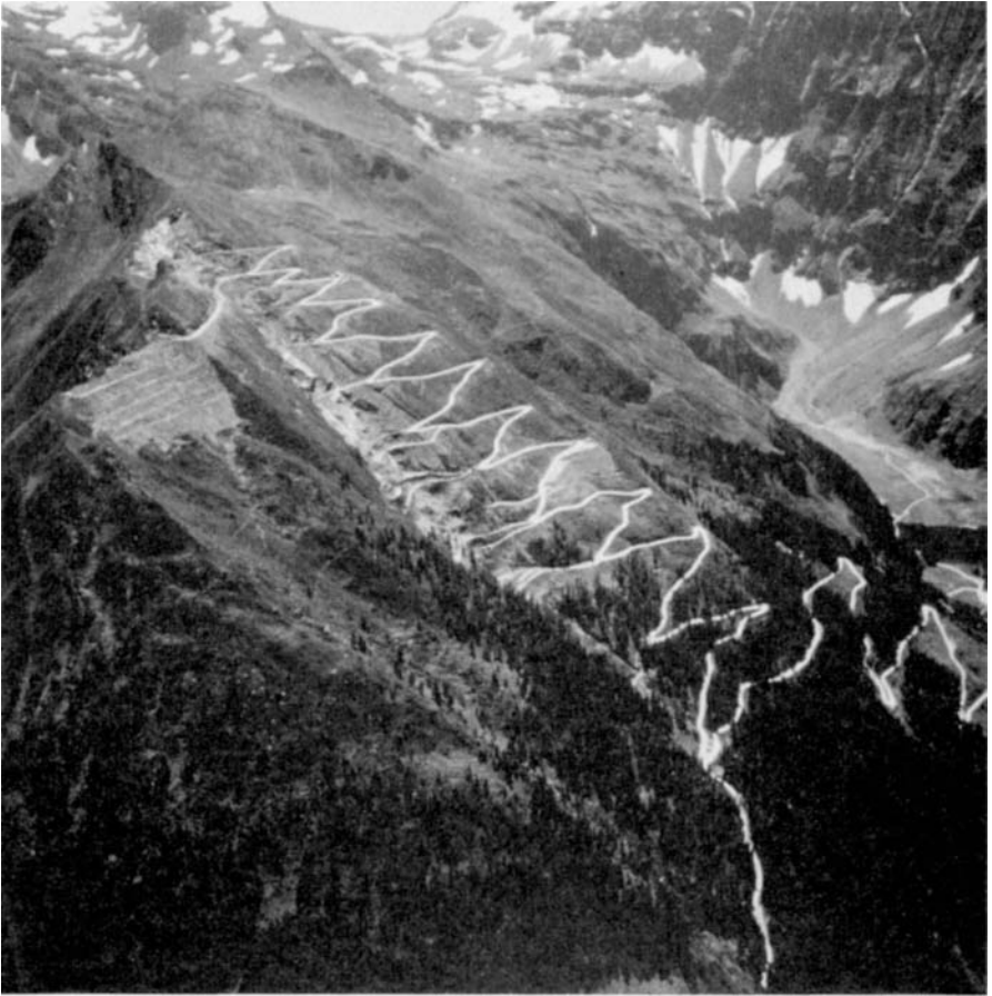
FIGURE 12.2. Specially constructed road to give access to the open pit mining area. By courtesy of Wolfram Bergbau und Hüttenges. m.b.H., Austria.
