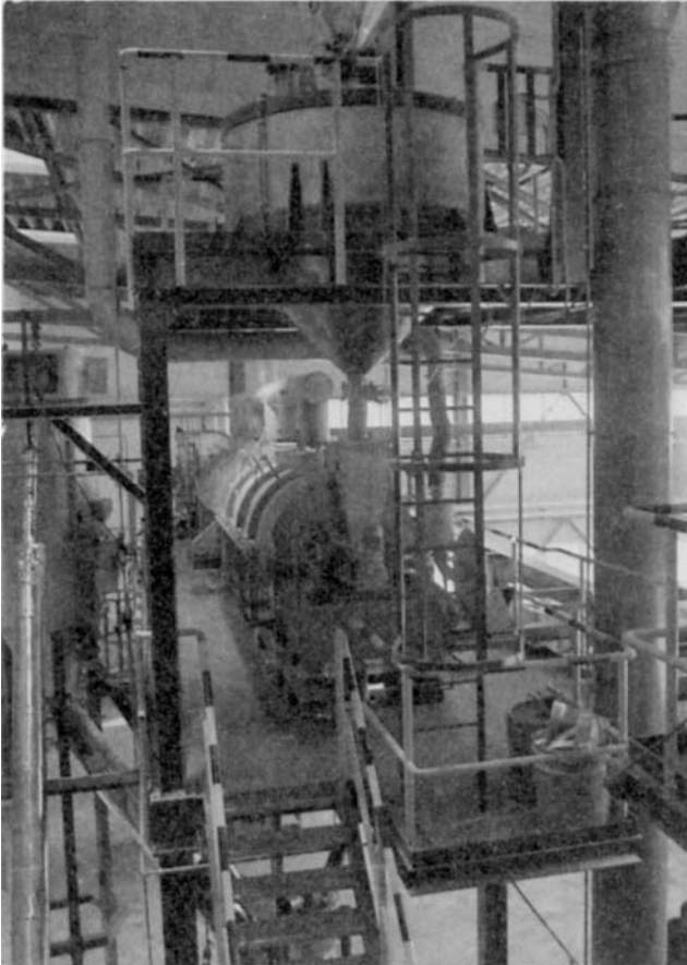
FIGURE 5.27. Rotary reduction furnace. By courtesy of Wolfram Bergbau- und Hüttenges. m.b.H., Austria.
