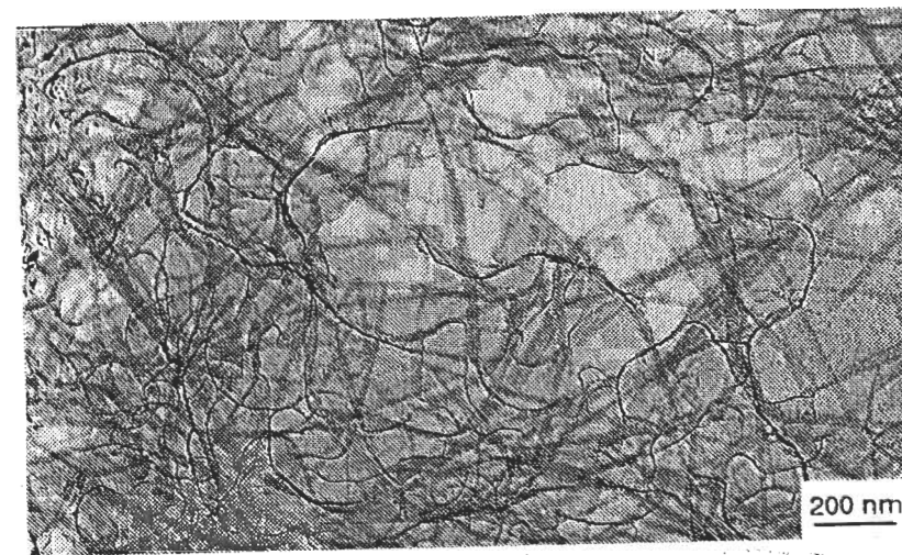
Figure 4.16 TEM micrograph of a vanadium oxide gel V 2 O 5 ·nH 2 O obtained via acidification of sodium metavanadate on an ion-exchange resin
