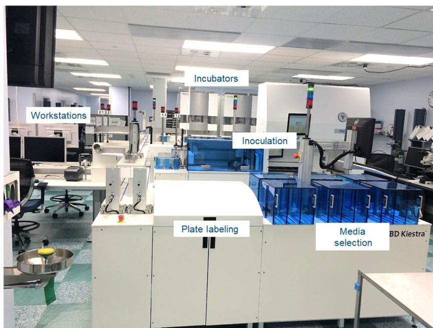
FIGURE 55.1 Components of total laboratory automation in clinical microbiology.
