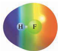
FIGURE 8.4 An electrostatic potential map of HF. Red indicates the most electron-rich area (the fluorine atom) and blue indicates the most electron-poor region (the hydrogen atom).
