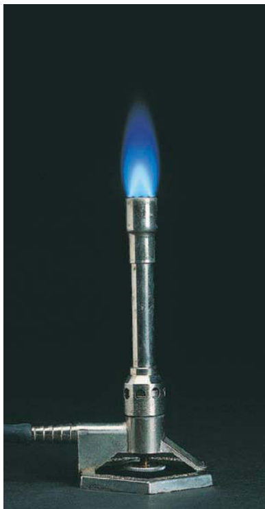
Methane reacts with oxygen to produce the flame in a Bunsen burner.
