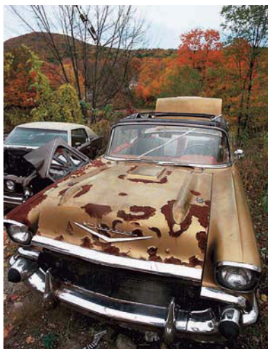
Formation of rust on bare steel is a spontaneous process.
