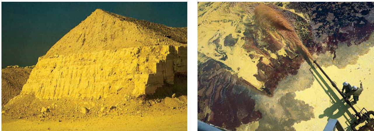
(left) A sulfur deposit. (right) Melted sulfur obtained from underground deposits by the Frasch process.
