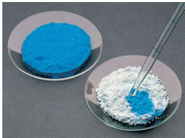
Hydrated copper(II) sulfate on the left. Water applied to anhydrous copper(II) sulfate, on the right, forms the hydrated compound.
