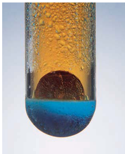
A copper penny reacts with nitric acid to produce \text{NO} gas, which is immediately oxidized in air to brown \text{NO}_2 .
