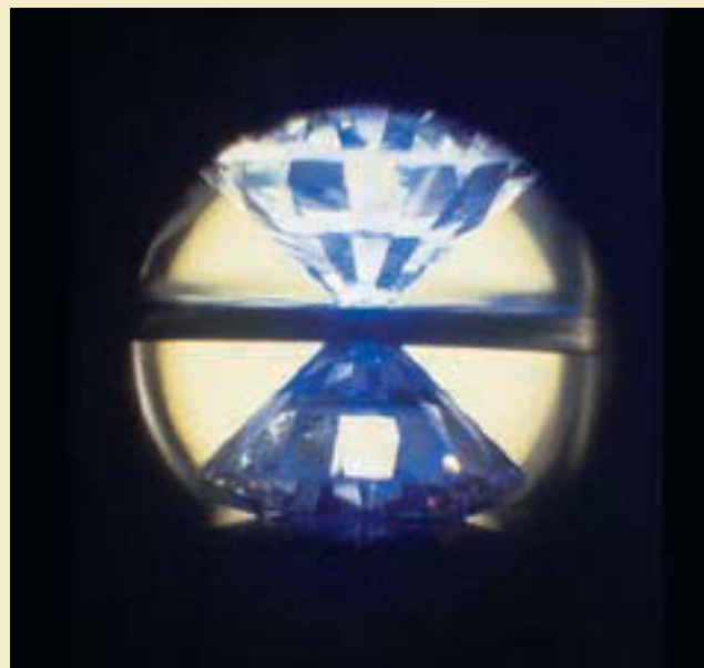
A diamond anvil cell used to study materials at very high pressures.
