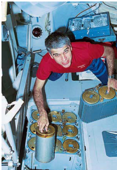
Astronaut Sidney M. Gutierrez changes the lithium hydroxide cannisters on space shuttle Columbia. The lithium hydroxide is used to purge carbon dioxide from the air in the shuttle's cabin.
