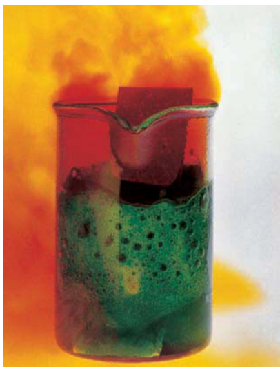
Oxidation of copper metal by nitric acid. The copper atoms lose two electrons to form \text{Cu}^{2+} ions, which give a deep green color that becomes turquoise when diluted with water.
