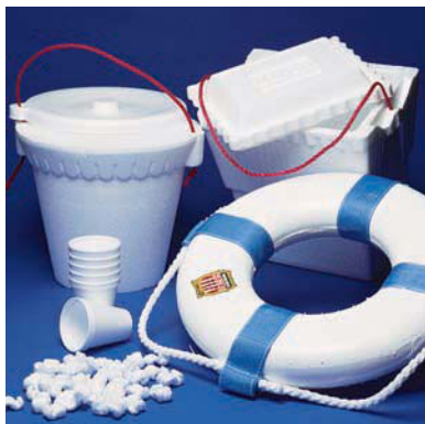
Blowing agents such as hydrazine, which forms nitrogen gas on decomposition, are used to produce porous plastics like these styrofoam products.
