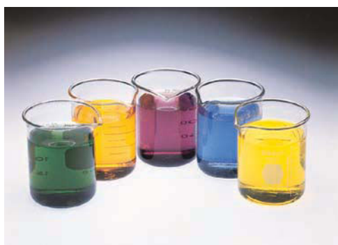
Various chromium compounds dissolved in water. From left to right: \text{CrCl}_2 , \text{K}_2\text{Cr}_2\text{O}_7 , \text{Cr}(\text{NO}_3)_3 , \text{CrCl}_3 , \text{K}_2\text{CrO}_4 .
