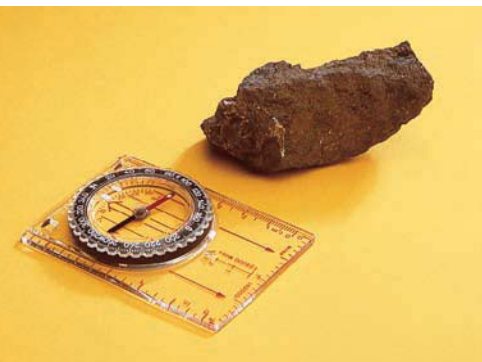
Magnetite is a magnetic ore containing \text{Fe}_3\text{O}_4 . Note that the compass needle points toward the ore.
