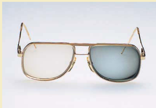
Glasses with photosensitive lenses. The right lens has been exposed to light and the left one has not.
