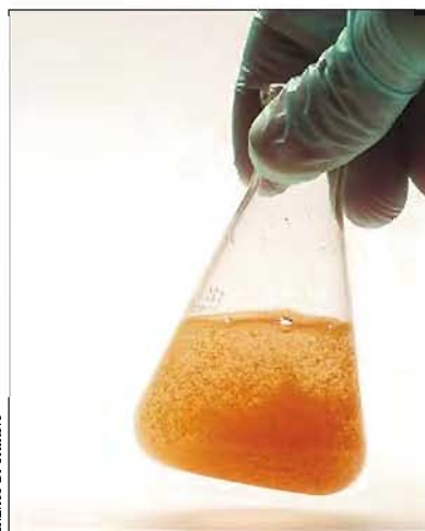
Figure 16.4 Titration of \text{Cl}^- with \text{Ag}^+ , using \text{CrO}_4^{2-} as an indicator. \text{AgCl} (cream color) comes down at first, then \text{Ag}_2\text{CrO}_4 (red) precipitates.
