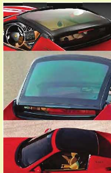
Figure A Reversible color changing electrochromic rooftop on the Ferrari Superamerica.
