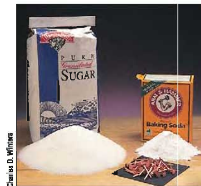
Figure 3.3 One-mole amounts of sugar (C 12 H 22 O 11 ), baking soda (NaHCO 3 ), and copper nails (Cu).
