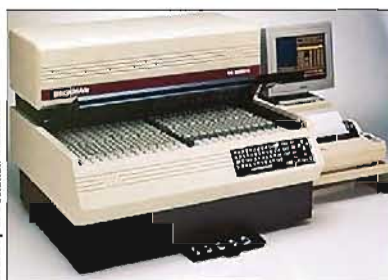
Figure 19.3 A liquid scintillation counter. This instrument is used to detect radiation and measure disintegrations per minute quickly and accurately.
