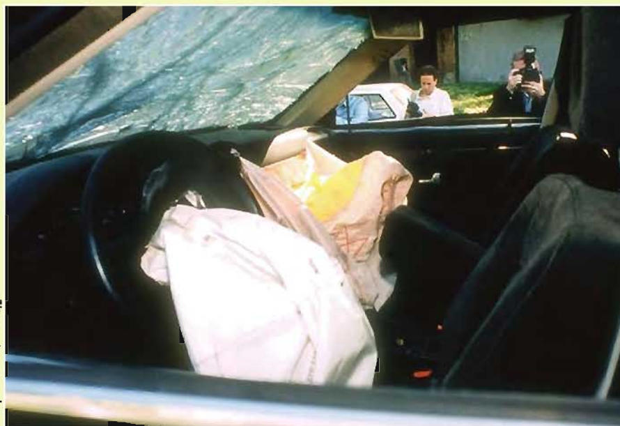
Figure A Deployed airbags after a collision are filled with nitrogen gas. The gas is a byproduct of the decomposition of sodium azide, which is triggered by the collision.
