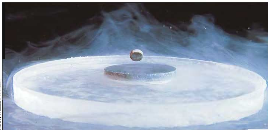
Figure 20.9 A superconductor. A pellet of superconducting material, previously cooled to 77 K with liquid nitrogen, floats above a magnet.
