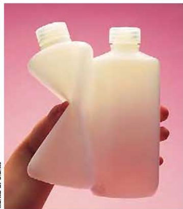
Figure 23.1 Branched and linear polyethylene. The polyethylene bottle at the left is made of pliable, branched polyethylene. The one at the right is made of semirigid, linear polyethylene.
