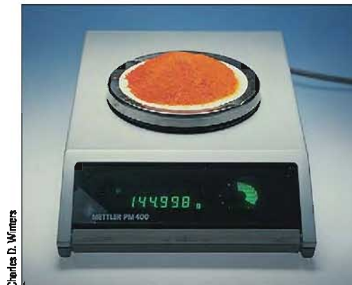
Figure 1.9 Weighing a solid. The solid sample plus the paper on which it rests weighs 144.998 g. The pictured balance is a single-pan analytical balance.
