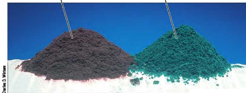
Figure 15.7 Cis and trans isomers of [\text{Co}(\text{en})_2\text{Cl}_2]^+ . The ethylenediamine molecule is represented by —en—. It forms two bonds per molecule. The cis isomer is reddish-purple and the trans is dark green.
