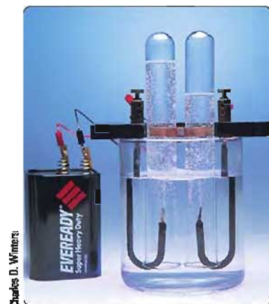
Figure 5.5 Electrolysis of water ( \text{H}_2\text{O} ). The volume of hydrogen ( \text{H}_2 ) formed in the tube at the right is twice the volume of oxygen ( \text{O}_2 ) formed in the tube at the left, in accordance with the equation 2\text{H}_2\text{O}(l) \longrightarrow 2\text{H}_2(g) + \text{O}_2(g) .
