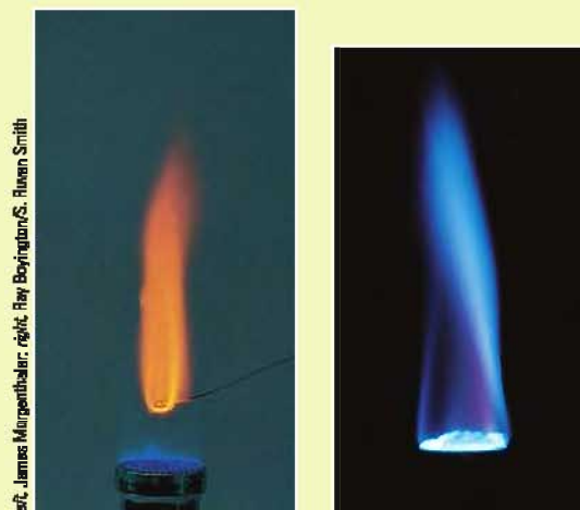
Figure C Flame tests for Na + (yellow) and K + (violet). A drop of solution is picked up on a platinum loop and immersed in the flame. The test for K + is best done with a filter that hides the strong Na + color.
