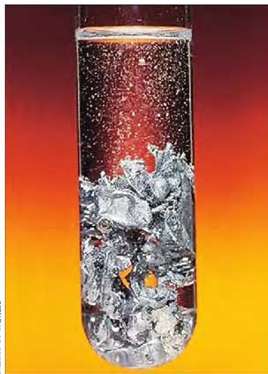
Figure 4.8 Redox reaction of zinc with a strong acid. The zinc atoms are oxidized to Zn 2+ ions in solution; the H + ions are reduced to H 2 molecules.
