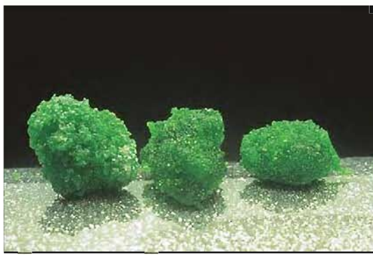
Figure 20.10 Oxidation of nickel. Nickel reacts slowly with hydrochloric acid to form \text{H}_2(\text{g}) and \text{Ni}^{2+} ions in solution. Evaporation of the solution formed gives green crystals of \text{NiCl}_2 \cdot 6\text{H}_2\text{O} .
