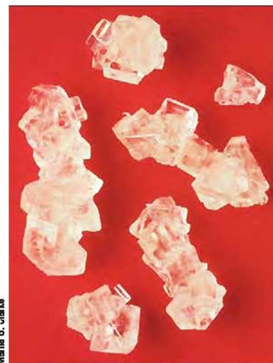
Figure 1.13 Rock candy. The candy is formed by crystallization of sugar from a saturated solution that is cooled slowly.
