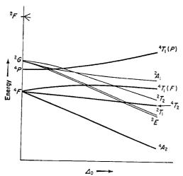
Fig. 25-C-1. Partial energy-level diagram for a  $d^3$  ion in an octahedral field (also for a  $d^7$ ion in a tetrahedral field). The quartet states are drawn with heavier lines.
