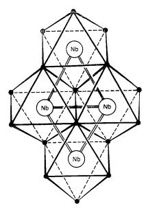
Fig. 26-B-6. The key structural unit in  $M^1Nb_4X_{11}$  compounds. Small filled circles are halogen atoms and double lines represent M—M bonds. Many of the peripheral halogen atoms are shared with other units.
