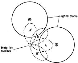
Fig. 20-36. A drawing of part of a complex, showing two lobes, A, A' of an  $e_g$  type metal orbital, two lobes, B, B' of a  $t_{2g}$  type metal orbital and two ligand atoms. The spheres enclosing most of the electron clouds of the ligand atoms are also shown.
