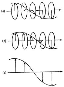
Fig. 20-20. (a) Right-circularly polarized light. (b) Left-circularly polarized light. (c) The plane-polarized resultant of (a) and (b). The horizontal arrow gives the direction of propagation, and the arrows perpendicular to this direction denote the instantaneous spatial direction of the electric vector. [Reproduced by permission from S. F. Mason, *Chem. in Britain*, 1965, 245.]
