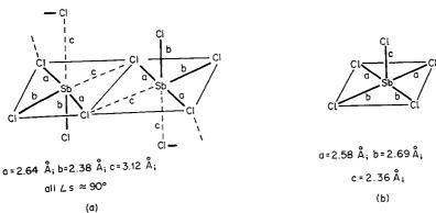
Fig. 13-5. (a) A portion of the anion chain in (pyH)SbCl<sub>4</sub>. (b) The SbCl<sub>5</sub><sup>2-</sup> ion found in (NH<sub>4</sub>)<sub>2</sub>SbCl<sub>5</sub>.
