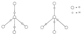
Fig. 5-7. Two possible configurations about an oxygen atom in ice.
