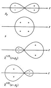
Fig. 3-4. Schematic illustration of the formation of sp digonal hybrid orbitals by combination of an s and a p orbital.
