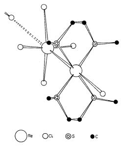
Fig. 26-D-10. The structure of Re<sub>2</sub>Cl<sub>5</sub>(DTH)<sub>2</sub>. The molecules form chains in the crystal and the dashed bond indicates a weaker intermolecular bond.
