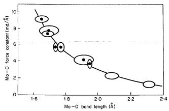
Fig. 3-21. Plot of bond lengths against force constant for Mo—O bonds (reproduced by permission from F. A. Cotton and R. M. Wing, *Inorg. Chem.*, 1965, 4, 867).
