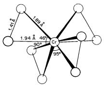
Fig. 25-C-4. The dodecahedral  $(D_{2d})$  structure of the  $CrO_8^{3-}$  ion.
