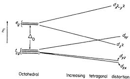
Fig. 20-6. Energy-level diagram showing the further splitting of the *d* orbitals as an octahedral array of ligands becomes progressively distorted by the withdrawal of two *trans*-ligands, specifically those lying on the *z*-axis.
