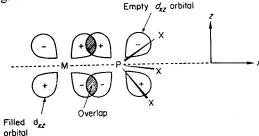
Fig. 22-17. Diagram showing the back-bonding from a filled metal d orbital to an empty phosphorus 3d orbital in the PX<sub>3</sub> ligand, taking the internuclear axis as the z-axis. An exactly similar overlap occurs in the yz plane using the  $d_{yz}$  orbitals.
