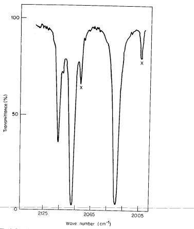
Fig. 22-12. The infrared spectrum of Rh<sub>2</sub>Cl<sub>2</sub>(CO)<sub>4</sub>. The small peaks marked X are <sup>13</sup>CO satellites. The large peaks are the three infrared-active fundamentals.
