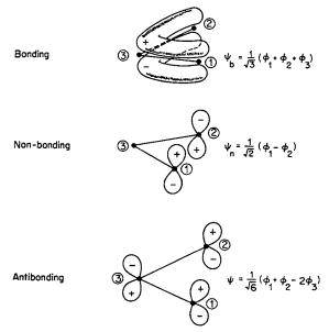
Fig. 3-15. Approximate shapes of the  $\pi$  MO's in nitrite ion, NO<sub>2</sub>.
