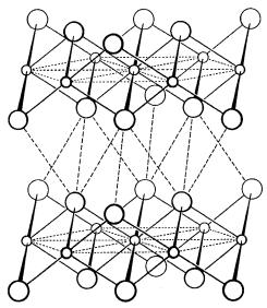
Fig. 2-4. A portion of the CdI<sub>2</sub> structure. Small spheres represent metal cations.
