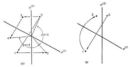
Fig. 1-5. Pictorial representations of the multiplication of symmetry operations. (a) Reflection times reflection. (b) Reflection followed by  $\mathbf{C}_3$ .
