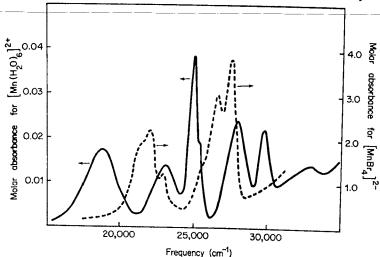
Fig. 20-17. The d-d absorption spectra of the  $[Mn(H_2O)_6]^{2+}$  ion (——, molar absorbance scale to the left) and the  $[MnBr_4]^{2-}$  ion (——, molar absorbance to the right).
