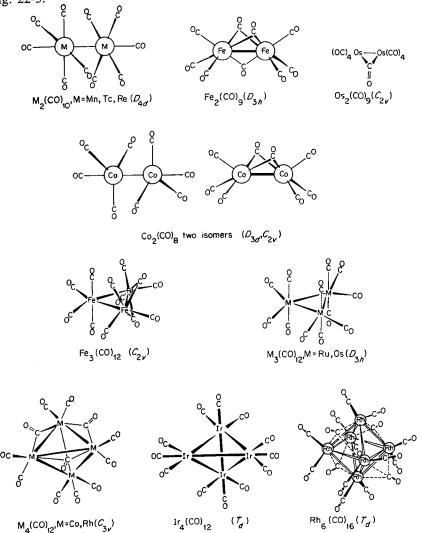
Fig. 22-3. The structures of some polynuclear metal carbonyls. The detailed structure of Os<sub>2</sub>(CO)<sub>9</sub> is not known.
