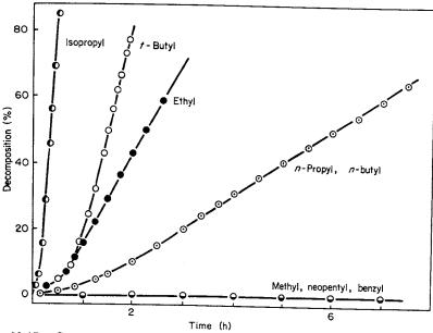
Fig. 23-17. Comparative rates of decomposition of dialkylmanganese in tetrahydrofuran at 2° (0.048M MnCl<sub>2</sub>, 0.27M Grignard reagent), the alkyl group being as stated in the diagram. [Reprinted by permission from M. Tamura and J. Kochi, J. Organometallic Chem., 1971, 29, 111.]
