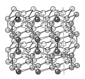
Fig. 5-6. The structure of ice I. Only the oxygen atoms are shown.
