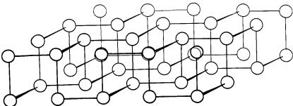
The arrangement of atoms in the double layers found in crystalline black phosphorus.
