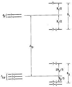
Fig. 20-28. Schematic diagram of the splittings caused by an elongation of an octahedron along one axis. The various splittings are not to the same scale,  $\delta_1$  and  $\delta_2$  being much smaller relative to  $\Delta_0$  than indicated.
