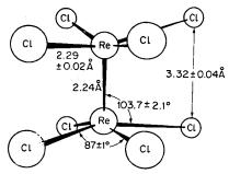
Fig. 26-D-5. The structure of the Re<sub>2</sub>Cl<sub>8</sub><sup>2-</sup> ion.
