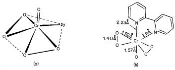
Fig. 25-C-3. The structures of (a)  $CrO(O_2)_2$  py and (b)  $CrO(O_2)_2$  bipy. The coordination polyhedron of (a) is approximately a pentagonal pyramid with the oxide oxygen at the apex.
