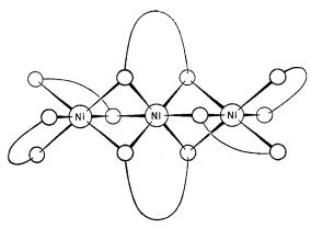
Fig. 25-G-2. Sketch indicating the trimeric structure of nickel acetylacetonate. The unlabelled circles represent oxygen atoms, and the curved lines connecting them in pairs represent the remaining portions of the acetylacetonate rings. [Reproduced by permission from J. C. Bullen, R. Mason and P. Pauling, *Inorg. Chem.*, 1965, 4, 456.]
