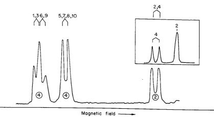
Fig. 8-9. The  $^{11}B$  nuclear magnetic resonance spectrum of  $B_{10}H_{14}$ . The assignment is shown at the top; circled numbers give intensities of the multiplets. The inset shows the appearance of a portion of the spectrum of 2-iodo- $B_{10}H_{13}$ .
