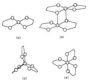
Fig. 22-18. The four basic structure types for "pure" dithiolene complexes: (a) square coordination; ( $D_{2h}$  molecular symmetry); (b) five-coordinate dimer; (c) trigonal-prismatic coordination ( $D_{3h}$  symmetry); (d) octahedral-coordination ( $D_3$  symmetry).
