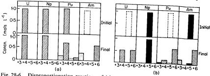
Fig. 28-6. Disproportionation reactions of (a) tetra- and (b) penta-positive ions in 1M acid at 25°. [Reproduced by permission from J. J. Katz and G. T. Seaborg, The Chemistry of the Actinide Elements, Methuen, London, 1957.]
