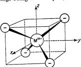
Fig. 20-5. Sketch showing the tetrahedral arrangement of four negative charges around a cation,  $M^{m+}$ , with respect to coordinate axes that may be used in identifying the d orbitals.
