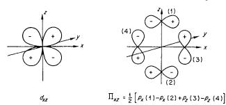
Fig. 20-40. At the right is the symmetry orbital, made up of ligand p orbitals, that has the proper symmetry to give optimum interaction with the metal ion  $d_{xz}$  orbital shown at the left. There are analogous symmetry orbitals,  $\pi_{xy}$  and  $\pi_{yz}$ , that are similarly related to the metal ion  $d_{xy}$  and  $d_{yz}$  orbitals.
