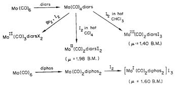
Fig. 26-C-12. Preparation of some carbonyl-containing molybdenum arsine and phosphine complexes.
