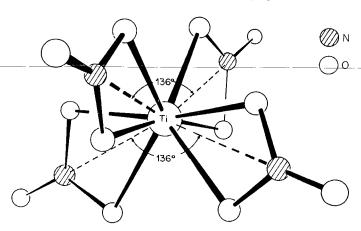
Fig. 25-A-2. The structure of titanium( $_{1}$ V) nitrate. Each NO<sub>3</sub> group is bidentate and they are disposed so that the N atoms form a slightly distorted tetrahedron with  $D_{2d}$  symmetry. [Reproduced by permission from C. D. Garner and F. C. Wallwork, J. Chem. Soc., A, 1966, 1496.]
