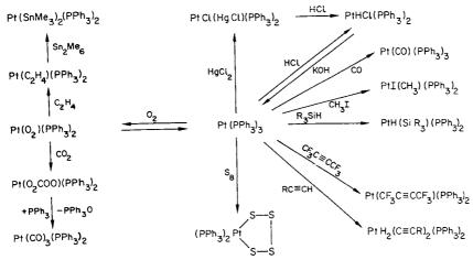
Fig. 26-H-3. Oxidative-addition and related reactions of tris(triphenylphosphine)platinum. Reactions with Pt(PPh<sub>3</sub>)<sub>4</sub> and the corresponding palladium complexes are similar.
