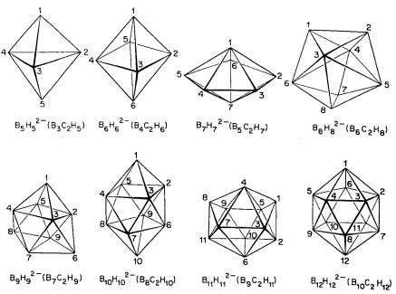
Fig. 8-10. The triangulated-polyhedral structures of  $B_nH_n^2$  and  $B_{n-2}C_2H_n$  species with the conventional numbering schemes also indicated.
