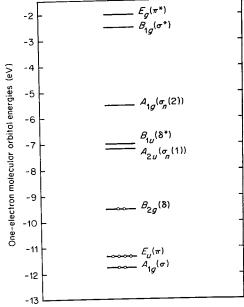
Fig. 19-10. An energy-level diagram for the MO's involved in Re—Re bonding in Re<sub>2</sub>Cl<sub>8</sub><sup>2-</sup>.
