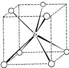
Fig. 26-A-2. Coordination geometry in the baddeleyite form of ZrO<sub>2</sub>.
