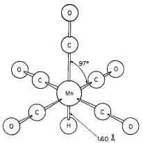
Fig. 22-16. The structure of the HMn(CO)<sub>5</sub> molecule, showing both the stereochemical activity of the hydrogen atom and the metal-to-hydrogen distance which approximates to the sum of normal covalent radii.
