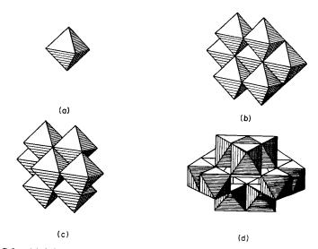
Fig. 26-C-2. (a) Diagrammatic representation of  $MoO_6$  and  $WO_6$  octahedra used in showing structures of some isopoly and heteropoly anions. (b) The structure of the paramolybdate anion,  $[Mo_7O_{24}]^6$ . (c) The structure of the octamolybdate anion,  $[Mo_8O_{26}]^4$  (note that one  $MoO_6$  octahedron is completely hidden by the seven that are shown). (d) The structure of the  $[W_{12}O_{42}]^{12}$  unit in the paratungstate ion.
