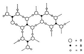
Fig. 5-2. The structure of boric acid showing hydrogen bonds.
