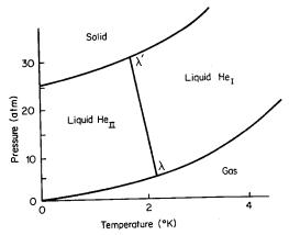
Fig. 17-1. Helium phase diagram near absolute zero.
