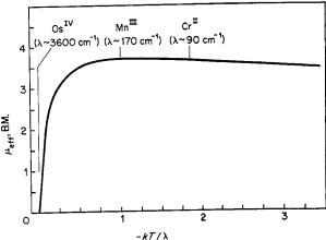
Fig. 26-1. Curve showing the dependence on temperature and on the spin-orbit coupling constant,  $\lambda$ , of the effective magnetic moment of a  $d^4$  ion in octahedral coordination.
