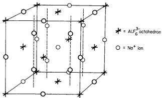
Fig. 9-2. The cubic structure of cryolite, Na<sub>3</sub>AlF<sub>6</sub>.
