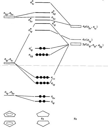
Fig. 23-8. An approximate MO diagram for ferrocene. Different workers often disagree about the exact order of the MO's; the order shown here, especially for the antibonding MO's, may be incorrect in detail, but the general pattern is widely accepted.
