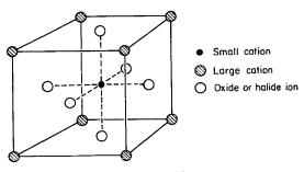
Fig. 2-5. The perovskite structure.
