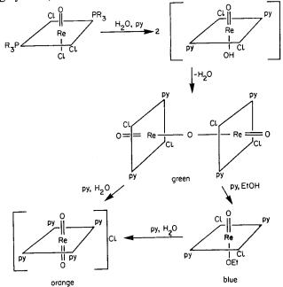
Fig. 26-D-8. Reaction of ReOCl<sub>3</sub>(PPh<sub>3</sub>)<sub>2</sub> with water and pyridine.
