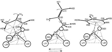
Fig. 23-21. Interconversion of the *syn*- and *anti*-proton at C-3 via a σ-allyl form (either transition state or intermediate). Obviously the same process occurs also at C-1. [Reproduced by permission from K. Vrieze and H. C. Volger, *J. Organometallic Chem.*, 1967, 9, 537.]
