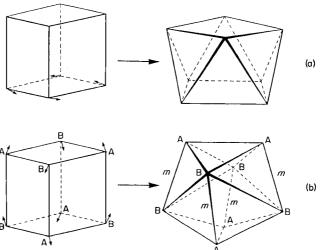
Fig. 1-10. The two most important ways of distorting the cube: (a) to produce a square antiprism; (b) to produce a dodecahedron.
