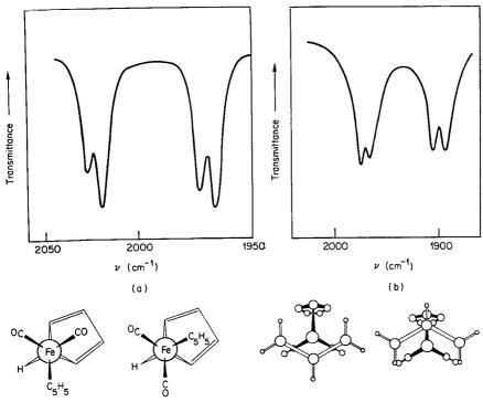
Fig. 22-13. Infrared spectra that demonstrate the presence of conformational isomers. (a) For the molecule  $(h^5-C_5H_5)$ Fe $(CO)_2(h^1-C_5H_5)$ ; data from F. A. Cotton and T. J. Marks, J. Amer. Chem. Soc., 1969, 91, 7523. (b) For the molecule  $(h^5-C_5H_5)$ Mo $(CO)_2C_3H_5$ ; data from R. B. King, Inorg. Chem., 1966, 5, 2242, and A. Davison and W. C. Rode, Inorg. Chem., 1967, 6, 2124.
