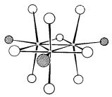
Fig. 19-6. The structure of  $Re_3X_9L_3$  molecules. The small circles represent rhenium atoms; the hatched circles represent L groups; the large open circles represent the X groups.
