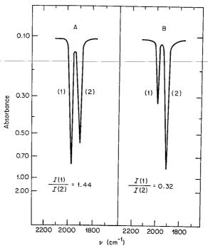
Fig. 22-10. The CO stretching bands and their relative intensities for the two cations of Figure 22-11. Data from F. A. Cotton and C. M. Lukehart, J. Amer. Chem. Soc., 1971, 93, 2672, and unpublished work,
