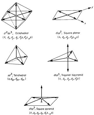
Fig. 3-6. Five important hybridization schemes involving d orbitals. Heavy arrows show the directions in which the lobes point.
