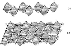
Fig. 9-3. Diagrams showing how AlF<sub>6</sub><sup>3</sup> octahedra combine by sharing corners in the compounds (a) Tl<sub>2</sub>AlF<sub>5</sub> and (b) NH<sub>4</sub>AlF<sub>4</sub>.
