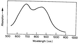
Fig. 20-29. The absorption spectrum of the  $[CoF_6]^{3-}$  ion in  $K_2Na[CoF_6]$ , showing the splitting due to a Jahn-Teller distortion of the excited state with the configuration  $t_{2g}^3e^3$ .
