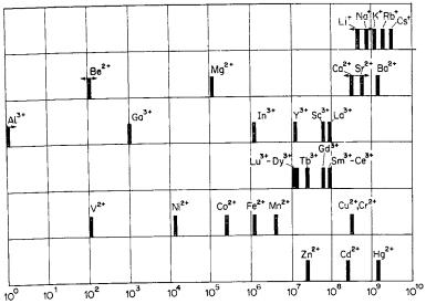
Fig. 21-9. Characteristic rate constants (sec<sup>-1</sup>) for substitutions of inner sphere H<sub>2</sub>O of various aquo ions. [Adapted from M. Eigen, *Pure Appl. Chem.*, 1963, 6, 105, with revised data kindly provided by M. Eigen. See also H. D. Bennett and B. F. Caldin, *J. Chem. Soc.*A, 1971, 2198.]
