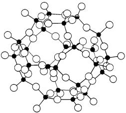
Fig. 11-5. The arrangement of AlO<sub>4</sub> and SiO<sub>4</sub> tetrahedra which gives the cubo-octahedral cavity in some zeolites and felspathoids. • represents Si or Al.
