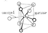
Fig. 26-D-11. The structure of ReH3<sup>-</sup>; the Re—H distance of 1.68 Å is consistent with the sum of single bond radii (Re = 1.28 Å).
