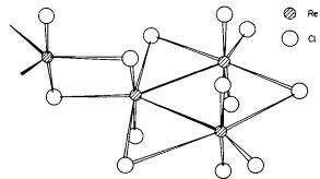
Fig. 26-D-3. The structure of Re<sub>3</sub>Cl<sub>9</sub>, showing how the trinuclear molecules are linked by chlorine bridges.
