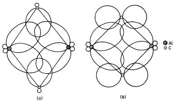
Fig. 10-6. Schematic indication of orbital overlaps in Al—C—Al bridge bonding. (a) For a methyl bridge. (b) Possible  $\pi$  component in phenyl bridging.
