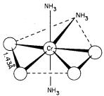
Fig. 25-C-5. The pentagonal bipyramidal structure of (NH<sub>3</sub>)<sub>3</sub>CrO<sub>4</sub>.
