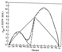
Fig. 27-2. Measured and calculated effective magnetic moments (BM) of lanthanide M<sup>3+</sup> ions at 300°K. I's are ranges of experimental values; —— gives values calculated for appropriate J ground states with allowance for the Sm and Eu anomalies; ---- gives values calculated without allowance for the Sm and Eu anomalies; ---- gives calculated spin-only values.
