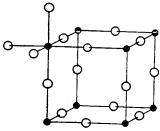
Fig. 26-D-2. The ReO<sub>3</sub> structure. Each metal atom lies at the center of an octahedron of oxygen atoms. This structure is closely related to the perovskite structure (page 55) since the latter is obtained from this one by insertion of a large cation in the center of the cube shown.
