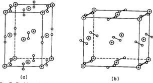
Fig. 10-3. The CaC<sub>2</sub> (a) and ThC<sub>2</sub> (b) structures (the latter is somewhat simplified here).
