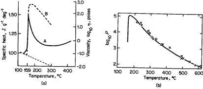
Fig. 15-2. (a) Specific heat (A) and viscosity (B) of liquid sulfur. (b) Chain length (P) as a function of temperature, × from magnetic susceptibility measurements and ☐ from esr measurements. [Reproduced by permission from Elemental Sulfur—Chemistry and Physics, B. Meyer, ed., Interscience, 1965.]
