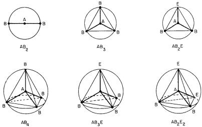
Fig. 4-1. Diagrams showing how the shapes of molecules are predicted when the valence shell of the central atom contains 2, 3 or 4 electron pairs.
