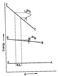
Fig. 20-19. Diagram showing how band width is related to the slope of the upper state relative to that of the ground state. A-A gives the energy of the ground state, B-B, and C-C the energies of two upper states as functions of the ligand field strength,  $\Delta$ .  $\delta\Delta$  represents the range of variation of  $\Delta$  due to the ligand vibrations, and  $\delta\nu_B$  and  $\delta\nu_C$  are the widths of the bands due to the transitions  $A \rightarrow B$  and  $A \rightarrow C$ .
