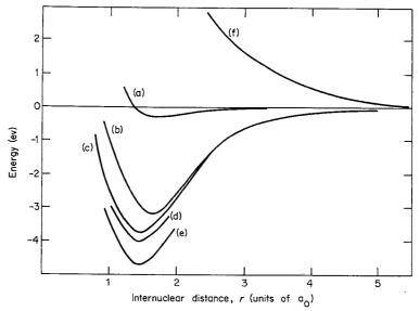
Fig. 3-1. Potential energy curves for the hydrogen molecule.
