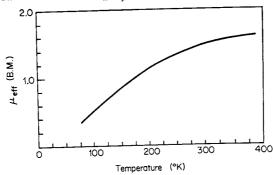
Fig. 25-H-6. Temperature-dependence of the effective magnetic moment per Cu atom in  $Cu_2(OCOCH_3)_4(H_2O)_2$ .
