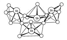
Fig. 13-7. The structure of the Sb<sub>4</sub>F<sub>16</sub><sup>4-</sup> ion in KSbF<sub>4</sub>.
