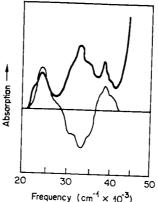
Fig. 20-26. The absorption spectrum (bold curve) and MCD spectrum (thinner curve) of  $K_3$ Fe(CN)<sub>6</sub> in the region of charge-transfer bands.
