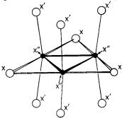
Fig. 26-D-4. A sketch of an isolated  $Re_3X_9$  unit which has  $D_{3h}$  symmetry. The three positions where additional ligands may be attached are indicated by  $X'' \rightarrow$ .
