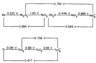
Fig. 26-D-1. Potential data for rhenium in basic solution (R. H. Busey, E. D. Sprague and R. B. Bevan, J. Phys. Chem., 1969, 73, 1039) and for technetium.
