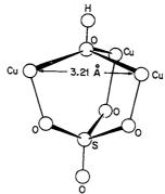
Fig. 25-H-7. Structural unit constituting the core of the compound  $Cu_3(C_6H_5N_2O)_3(OH)$  (SO<sub>4</sub>)·16.3H<sub>2</sub>O.
