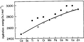
Fig. 20-30. Hydration energies of some divalent ions. Solid circles are experimentally derived hydration energies. Open circles are energies corrected for LFSE.
