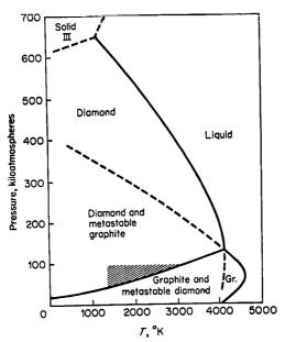
Fig. 10-1. Carbon phase diagram. Shaded area is the most favorable for catalyzed graphite-diamond conversion. [Adapted from F. P. Bundy, J. Chem. Phys., 1963, 38, 618, 631.]
