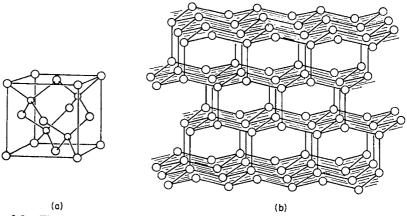
Fig. 2-8. The diamond structure seen from two points of view. (a) The conventional cubic unit cell. (b) A view showing how layers are stacked; these layers run perpendicular to the body diagonals of the cube.
