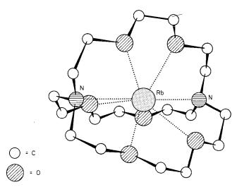
Fig. 6-1. The structure of the cation in the salt [RbC<sub>18</sub>H<sub>36</sub>N<sub>2</sub>O<sub>6</sub>]SCN·H<sub>2</sub>O. [Reproduced by permission from M. R. Truter, *Chem. in Britain*, 1971, 203.]
