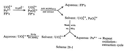
2. Tributyl phosphate method. The extraction coefficients from 6N nitric acid solutions into 30% tributylphosphate in kerosine are  $Pu^{4+} > PuO_2^{2+}$ ;  $Np^{4+} \sim NpO_2^+ \gg Pu^{3+}$ ;  $UO_2^{2+} > NpO_2^+ > PuO_2^{2+}$ ; the  $M^{3+}$  ions have very low extraction coefficients in 6M acid, but from 12M hydrochloric acid or 16M nitric acid the extraction increases and the order is Np < Pu < Am < Cm < Bk.
