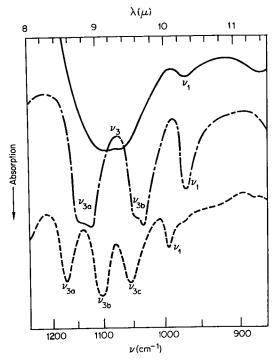
Fig. 21-7. Infrared spectra of  $[Co(NH_3)_6]_2(SO_4)_3 \cdot 5H_2O$  (——);  $[Co(NH_3)_5SO_4]$  Br (-·-·-);  $[(NH_3)_4 Co(\mu\text{-NH}_2) (\mu\text{-SO}_4) Co(NH_3)_4] (NO_3)_3 (---)$ . [Reproduced by permission from K. Nakamoto, ref. 28.]
