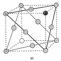
Fig. 2-2. (a) The stacking of close-packed layers in the ABC pattern which, on repetition, gives cubic closest packing, *ccp*. (b) Another view of the *ccp* pattern emphasizing its cubic symmetry.
