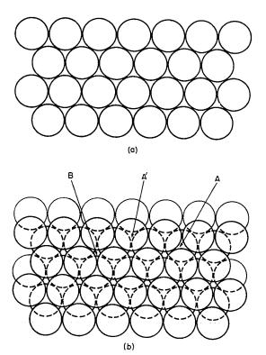
Fig. 2-1. (a) One close-packed layer of spheres. (b) Two close-packed layers showing how tetrahedral (A, A') and octahedral (B) interstices are formed.
