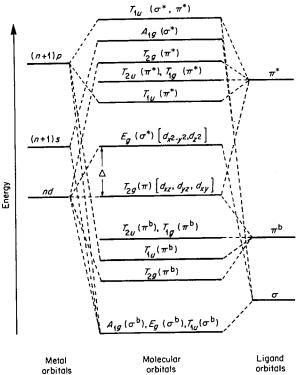
Fig. 20-42. A qualitative molecular orbital diagram for an M(CO)<sub>6</sub> or [M(CN)<sub>6</sub>]<sup>n</sup>-compound. [Adapted from H. B. Gray and N. A. Beach, *J. Amer. Chem. Soc.*, 1963, 85, 2922.]
