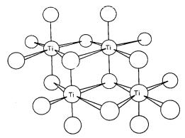
Fig. 25-A-1. The tetrameric structure of crystalline Ti(OC<sub>2</sub>H<sub>5</sub>)<sub>4</sub>. Only Ti and O atoms are shown.
