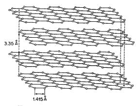
Fig. 10-2. The normal structure of graphite.
