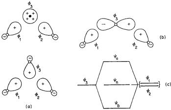
Fig. 3-16. Open 3-center bonding. (a) Two situations in which the central orbital,  $\phi_3$ , is symmetric. (b) The case where  $\phi_3$  is antisymmetric. (c) The type of energy level diagram that arises in either case (a) or case (b).
