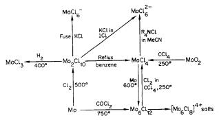
Fig. 26-C-8. Preparation of molybdenum chlorides and chloro complexes.
