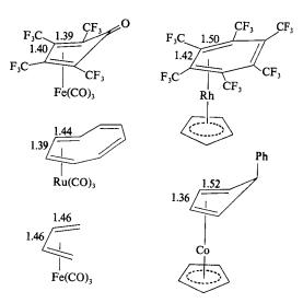
Fig. 23-4. Some structures in which butadiene units are bonded to metal atoms. The numbers give the average lengths, in Å, of the C-1/C-2 and C-3/C-4 bonds and the C-2/C-3 bond length, in each case.
