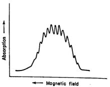
Fig. 20-34. The esr spectrum of the [IrCl<sub>6</sub>]<sup>2-</sup> ion, obtained with the applied magnetic field aligned along one of the Cl—Ir—Cl axes of the complex ion in a single crystal of Na<sub>2</sub>PtCl<sub>6</sub>·6H<sub>2</sub>O containing 0.5% of Ir<sup>IV</sup> substitutionally replacing Pt<sup>IV</sup>.
