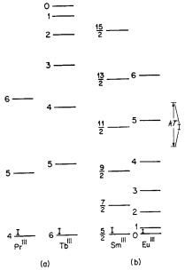
Fig. 27-1. J states for several lanthanides: (a) two of the several cases where the J states are widely separated compared to kT and (b) the two cases where the separations are of the same order as, or less than, kT.
