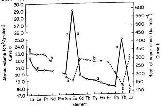
Fig. 27-3. The atomic volumes (curve a) and heats or vaporization (curve b) of the lanthanide metals.
