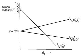
Fig. 25-D-1. Simplified energy level diagram for the  $d^4$  system,  $Mn^{III}$ , in octahedral surroundings.
