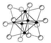
Fig. 26-B-5. The structure of the  $[M_6X_{12}]^{n+}$  units found in many halogen compounds of lower-valent niobium and tantalum. [Reproduced by permission from L. Pauling, *The Nature of the Chemical Bond*, 3rd edn., Cornell Univ. Press, 1960.]
