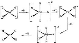
Fig. 21-13. Two-stage mechanism for the catalytic isomerization of cis-[Pd(amine)<sub>2</sub>X<sub>2</sub>] complexes to the corresponding trans-isomers.
