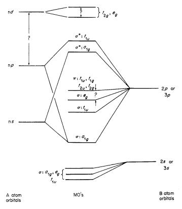
Fig. 4-7. A schematic molecular orbital energy diagram for an AB<sub>6</sub> molecule in which the center atom has ns, np, and nd valence-shell orbitals.
