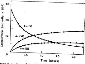
Fig. 28-5. Disproportionation of AmO<sup>+</sup><sub>2</sub> in 6M perchloric acid at 25°. Net reaction 3AmO<sup>+</sup><sub>2</sub> +4H<sup>+</sup>=2AmO<sup>+</sup><sub>2</sub> +Am<sup>3+</sup>+2H<sub>2</sub>O. [Reproduced by permission from J.S. Coleman, Inorg. Chem., 1963, 2, 53.]
