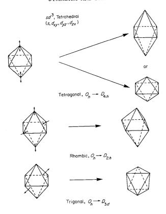
Fig. 1-9. Sketches showing the three principal types of distortion found in real octahedral complexes.
