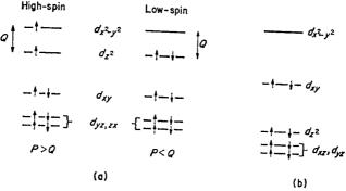
Fig. 20-12. Energy-level diagrams showing the possible high-spin and low-spin ground states for a  $d^8$  system (e.g., Ni<sup>2+</sup>) in a tetragonally distorted octahedral field. (a) Weak tetragonal distortion; (b) strong distortion or square field.
