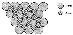
Fig. 8-1. Parallel layers of metal atoms and boron atoms in MB<sub>2</sub> compounds.
