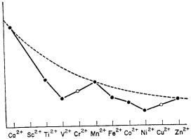
Fig. 20-27. The relative ionic radii of divalent ions of the first transition series. The broken line is a theoretical curve explained in the text.
