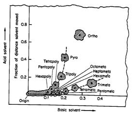
Fig. 13-13. Chromatographic separation of complex phosphate mixtures. Corner of a two-dimensional paper chromatogram, showing the positions of the pentameta-through octameta-phosphate rings in relation to the positions of the well known ring and chain phosphates. The basic solvent traveled 23 cm in 24 h, whereas the acid solvent traveled 11.5 cm in 5.5 h.
