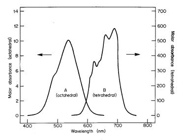
Fig. 25-F-4. The visible spectra of  $[Co(H_2O)_6]^{2+}$  (curve A) and  $[CoCl_4]^{2-}$  (curve B). The molar absorbance scale at the left applies to curve A, and that at the right applies to curve B.
