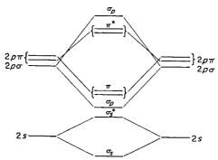
Fig. 3-13. The energy level diagram obtained in a molecular orbital treatment of a homonuclear diatomic molecule in which only s and p orbitals are used and  $s\sigma-p\sigma$  interactions are neglected.
