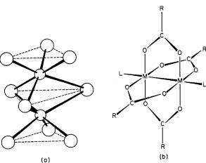
Fig. 19-5. Two types of structure in which a full range of M—M interaction from strongly bonding to net repulsive can be observed. (a) The confacial bioctahedron. (b) The carboxylato-bridged dinuclear molecules.
