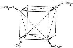
Fig. 25-E-3. The four iron atoms and four "inorganic" sulfur atoms in HiPIP form an eight-atom polyhedra of the type 1-XLVII (page 33). A tetrahedral set of sulfur atoms around each iron atom is completed by cysteine-sulfur atoms.
