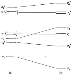
Fig. 3-14. The effect of  $s\sigma-p\sigma$  interactions on the level order in a homonuclear diatomic molecule: (a) is the level order transcribed from Fig. 3-13; (b) is the level order after appreciable  $s\sigma-p\sigma$  interaction is introduced.
