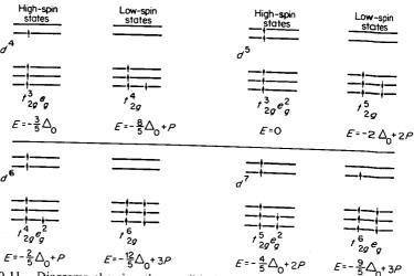
Fig. 20-11. Diagrams showing the possible high-spin and low-spin ground states for  $d^4$ ,  $d^5$ ,  $d^6$  and  $d^7$  ions in octahedral crystal fields, including the notation for writing out the configurations and expressions for their energies, derived as explained in the text.
