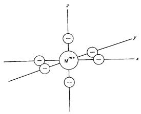
Fig. 20-1. Sketch showing six negative charges arranged octahedrally around a central  $M^{m+}$  ion with a set of Cartesian axes for reference.
