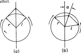
Fig. 20-21. (a) An instantaneous view along the direction of propagation of the two vectors r and l of the circularly polarized beams and their resultant which lies in a vertical plane. (b) If  $n_l > n_r$ , the beam l is retarded relative to beam r, thus causing the plane of the resultant to be tilted by the angle  $\alpha$ .
