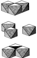
Fig. 26-C-4. An exploded view of the structure of the 9-molybdoheteropoly anion  $[X^{n+}Mo_9O_{32}]^{(10-n)-}$ , showing the nine  $MoO_6$  octahedra. When the upper and lower sets of three are moved in so as to share some corners with the equatorial set, a central octahedron of oxygen atoms occupied by the hetero atom is created.
