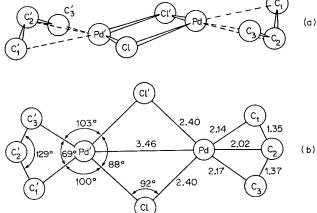
Fig. 23-16. Structure of allylpalladium(II) chloride dimer. Bond lengths are in Å. [Reprinted by permission from J. Organometallic Chem., 1965, 3, 43.]
