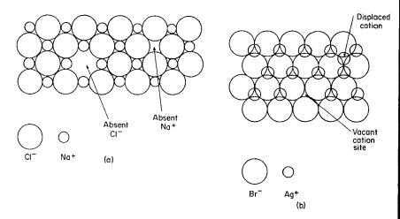
Fig. 2-14. (a) A Schottky defect in a layer of NaCl. (b) A Frenkel defect in a layer of AgBr. The defects need not be restricted to one layer, as shown here.
