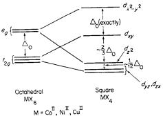
Fig. 20-7. Approximate energy-level diagram for corresponding octahedral and square complexes of some metal ions in the first transition series.
