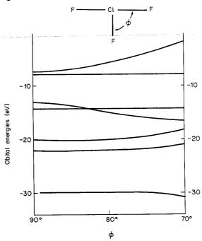
Fig. 4-6. Orbital energies (eV) as a function of angle for CIF<sub>3</sub> as calculated in the extended Hückel approximation. [Adapted from Gavin.<sup>5</sup>]
