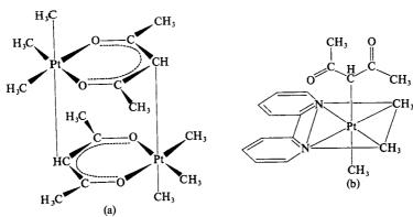
Fig. 26-H-2. (a) The molecular structure of trimethylplatinum acetylacetonate dimer, showing how the Pt<sup>IV</sup> attains octahedral coordination. (b) Schematic representation of the molecular structure of the bipyridine adduct of trimethylplatinum(IV) acetylacetonate.
