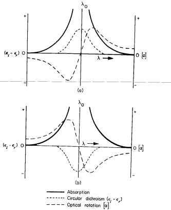
Fig. 20-23. The Cotton effect, as manifested in circular dichroism,  $\varepsilon_l - \varepsilon_r$ , and optical rotatory dispersion,  $[\alpha]$ , as would be given by a dissymmetric compound with an absorption band centered at  $\lambda_0$ , on the assumption that there are no other absorption bands close by. (a) A positive Cotton effect. (b) A negative Cotton effect.
