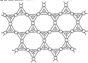
Fig. 11-4. Sheet silicate anion structure idealized. [For a real example see A. K. Pant Acta Cryst., B, 1968, 24, 1077.]
