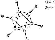
Fig. 25-H-2. The Cu<sub>6</sub>P<sub>6</sub> group in [CuH(PPh<sub>3</sub>)]<sub>6</sub>. The Cu—Cu distances shown as full lines have an average value of 2.65 Å while those shown by broken lines average 2.54 Å.
