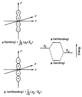
Fig. 20-38. To the left are orbital pictures showing the bonding and antibonding molecular orbitals that are the z components of the  $T_{1u}$  sets. To the right is an energy-level diagram showing how the energies of the various orbitals are related.
