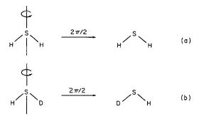
Fig. 1-1. Sketches showing that the operation  $C_2$  carries  $H_2S$  into an orientation indistinguishable from the original, but HSD into an observably different orientation.
