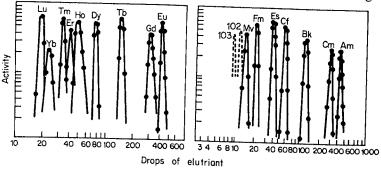
Fig. 28-7. Elution of lanthanide +3 ions (left) and actinide +3 ions (right) from Dowex 50 cation-exchange resin. Buffered ammonium 2-hydroxybutyrate was the cluant. The predicted positions of elements 102 and 103 (unobserved here) are shown by broken lines. [Reproduced by permission from J. J. Katz and G. T. Seaborg, The Chemistry of the Actinide Elements, Methuen, London, 1957.]
