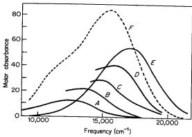
Fig. 25-H-5. Absorption spectra of  $[Cu(H_2O)_6]^{2+}$  (A) and of the ammines in 2M ammonium nitrate at 25°,  $[Cu(NH_3)(H_2O)_5]^{2+}$  (B),  $[Cu(NH_3)_2(H_2O)_4]^{2+}$  (C),  $[Cu(NH_3)_3(H_2O)_3]^{2+}$  (D),  $[Cu(NH_3)_4(H_2O)_2]^{2+}$  (E), and  $[Cu(NH_3)_5H_2O]^{2+}$  (F).
