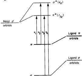
Fig. 20-46. Partial MO diagram for an octahedral  $MX_6$  complex, showing the four main classes of  $L\rightarrow M$  charge-transfer transitions.
