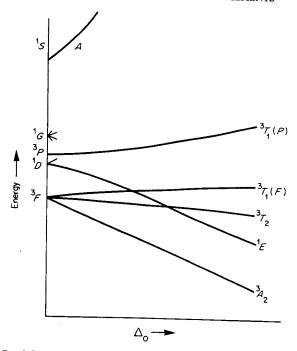
Fig. 20-16. Partial energy-level diagram for a  $d^8$  ion in an octahedral field, showing the triplet states and only the lowest singlet state.
