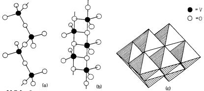
Fig. 25-B-2. Structures in the crystalline state of anions in (a) KVO<sub>3</sub>, (b) KVO<sub>3</sub>·H<sub>2</sub>O, and (c) decayanadates,  $[V_{10}O_{28}]^{16}$ .
