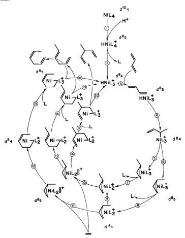
Fig. 24-B-3. Catalytic cycle for the formation of 1,4-hexadiene from ethylene and butadiene by use of nickel complexes. The numbers 4 or 5 after the electron configurations denote the coordination number of the species. [Reproduced by permission from a diagram provided by Dr. C. A. Tolman, Central Research Laboratory, E. I. du Pont de Nemours and Co., and published in J. Amer. Chem. Soc., 1970, 92, 6777].
