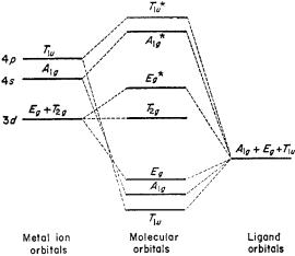
Fig. 20-39. The molecular orbital energy-level diagram, qualitative, for an octahedral complex between a metal ion of the first transition series and six ligands that do not possess  $\pi$  orbitals.
