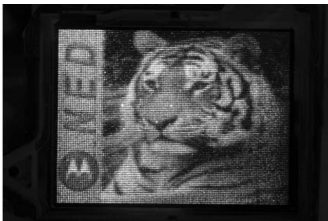
Fig. 6.19 A colour field emission display using carbon nanotubes, developed by Motorola Labs.
