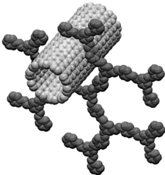
Fig. 8.9 Model of stilbenoid dendrimer wrapped around a (10, 10) nanotube (8.60).
