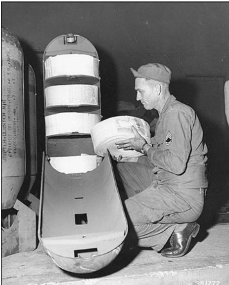
Figure 16.2. A soldier loading an M-16-A1 bomb, capable of holding 22,500 eight-by-five-inch leaflets. During the Korean War, a B-29 would normally carry 32 of these bombs, each of which weighed 170 pounds, and drop them from an altitude of about 20,000 feet. At 1,000 feet above the ground, a fuse opened the device and spread the leaflets. By early December 1950, the Far Eastern Air Force had disseminated 147 million leaflets—or millions of insects—using these devices. (Courtesy of Ed Rouse)
