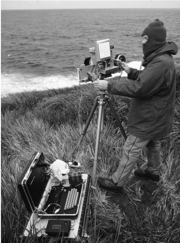
FIGURE 15.2 The author tracking albatrosses and petrels with the original ornithodolite at Bird Island, South Georgia in January 1980. The observer looks through the rangefinder eye piece (upper right) while steering the instrument with the handle at right to keep it aligned on the bird, and rotating the handle at left to set the rangefinder. Pressing the white button (by right thumb) captured an observation of the bird's azimuth, angular altitude and range, together with the time. The large dial by the observer's right hand is a display of wind speed and direction, coming from a yacht anemometer head, mounted on a mast a few metres away. Data on species and wind were entered with the keyboard and the whole record was recorded on a cassette tape recorder (nearest camera). Photo by J.P. Croxall.
