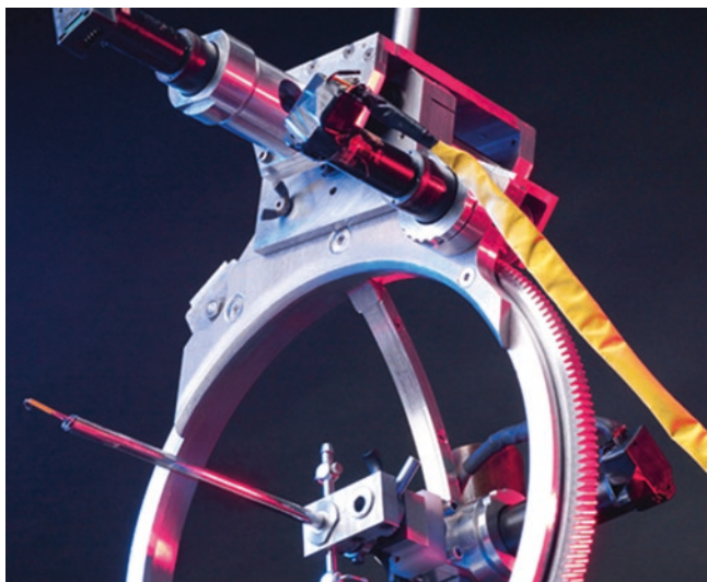
Fig. 1.3 The PROBOT was able to performed precise and repetitive cone shaped cuts of the prostate following an pre-establish plan
