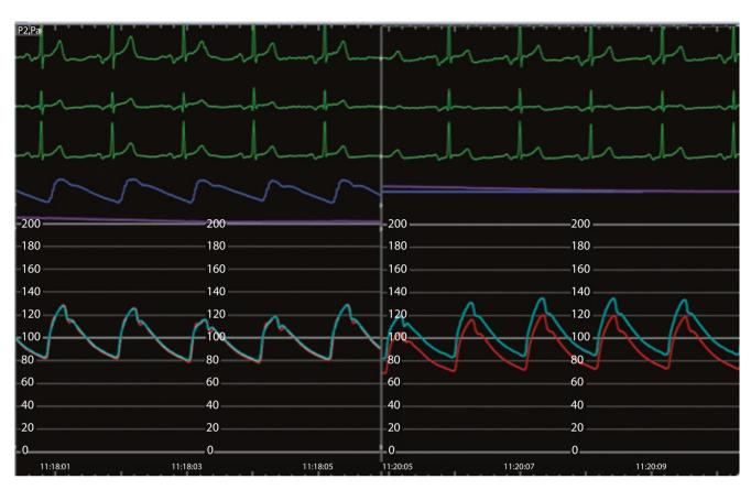
■ Fig. 10.10 Loose connections. Equalized  $P_a$  and  $P_d$  pressures (*left panel*) become unequal when the Touhy-Borst introducer is not tightened (*right panel*), causing partial loss of aortic pressure. Leaving a needle introducer in place causes a similar loss of pressure
