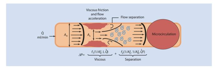
■ Fig. 14.2 Total pressure loss derives from two sources: frictional losses along the entrance and throat and inertial losses stemming from the sudden expansion, causing flow separation and eddies (exit losses). Frictional losses are linearly related to flow, *Q* (law of Poiseuille), and exit losses increase with the square of the flow caused by convective accel-
