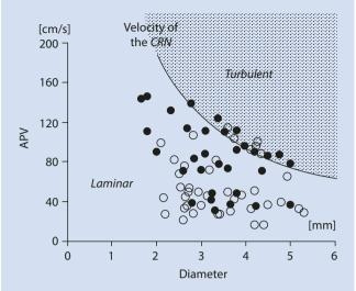
■ Fig. 10.7 Maximum value of the average peak velocity APV in 43 patients before (○) or after an angiographically successful angioplasty of 32 patients (●). The highest values of APV were taken for each individual. The flow velocity at the critical Reynolds number (CRN) 500 describes the change from laminar to turbulent flow profile (From Ferrari [9])
