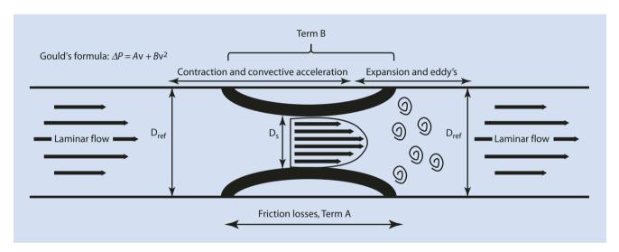
**□ Fig. 12.3** The total transstenotic pressure gradient ( $\Delta P$ ) is calculated by  $\Delta P = Av + Bv^2$ . At the entrance and along the throat of the stenosis, pressure is lost by frictional resistance and determined by the law of Hagen-Poiseuille, which is translated into term A. Contraction, with subsequent convective acceleration of flow along the throat of
