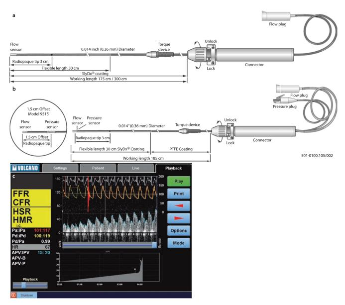
■ Fig. 11.2 Doppler flow velocity instrumentation. a FloWire (Volcano-Philips). A 0.014″ guide wire with a Doppler crystal at the tip. b ComboWire (Volcano-Philips). A 0.014″ guide wire equipped with both a Doppler crystal at the tip and a pressure sensor either just distal or at 1.5 cm distal to the Doppler crystal. c ComboMap console display. Instrumentation displays temporal changes in coronary flow velocity (Doppler signal in
