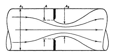
Fig. 3.13 Fluid flowing through a tube of diameter  $A_1$  approaches an orifice of diameter A. The fluid will continue to narrow to a minimal diameter at  $A_2$  somewhat distal to the orifice. It is this "effective valve area" at  $A_2$  and not the true anatomic area at the orifice, that is calculated using the continuity equation. The system's lowest pressure is also at  $A_2$  and not at the anatomic orifice.
