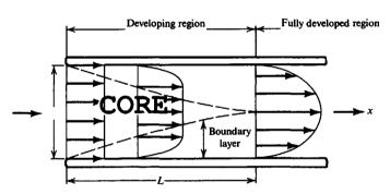
Fig. 3.3 As fluid enters a pipe it progresses along and will assume a parabolic shape. The length *L* is the *developing region* (unestablished flow), and when flow then becomes parabolic it is the *developed region* (established flow). The developing region will become dominated by the growth of the *boundary layer*, and a diminishing *core* of fluid at the center of the pipe. Established flow will result from
