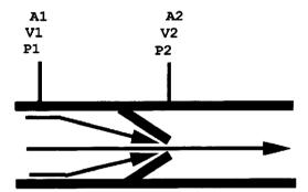
**Fig. 3.8** As fluid approaches a narrowing within a pipe it will accelerate  $(V_1 < V_2)$ . According to Bernoulli's law, in order that hydraulic energy remain constant at every point in the pipe, the pressure will necessarily decrease  $(P_1 > P_2)$ .  $A_1$  and  $A_2$  are cross-sectional areas at the respective locations along the pipe (see text).
