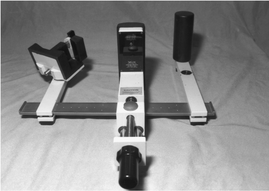
FIGURE 4.9. Telos pressure bar with LED digital readout. The force is applied by rotating the handle of the shaft up to 20 kiloponds.
