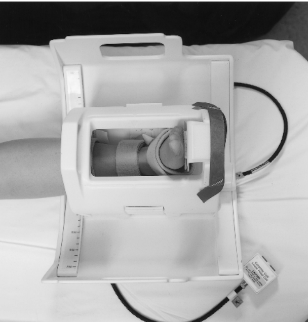
FIGURE 4.20. Custom built hindfoot positioning device for magnetic resonance imaging (MRI) scans. The device is worn while scanning is done inside the extremity coil.
