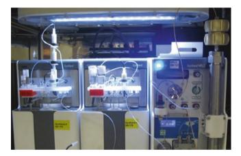
**Fig. 10.2** The latest generation of synthesis modules: *IBA SynthERA II* (*left* and *center*), *SynthERA HPLC* module (*right*)—a HPLC system
