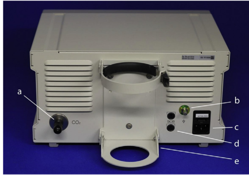
Figure 7.8 Gas insufflator, rear panel: a, gas inlet; b, ground connector; c, mains plug; d, SCB (STORZ Communication Bus) connector, bus system to transfer data to other peripheral devices; e, holder for small gas bottle if the insufflator is mounted on a trolley. From MITI.
