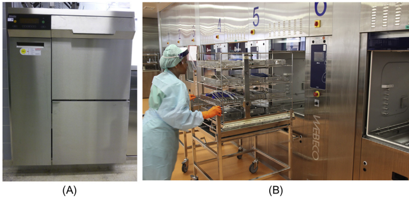
Figure 4.7 Modern instrument processing unit: (A) instrument washing machine in the OR; (B) washing machines in a central reprocessing and sterilization unit. All from MITI.
