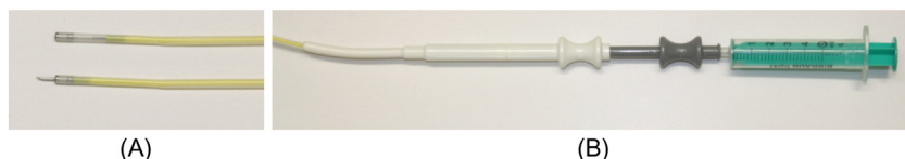
Figure 8.9 Injector needle: (A) Retracted (up) and locked in working position (below); (B) syringe connected to the external end of the probe. All from MITI.
