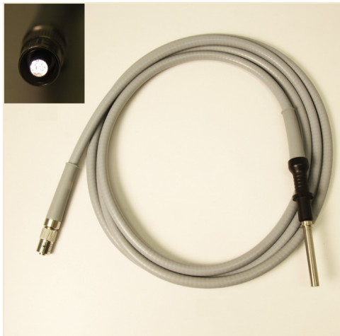
Figure 7.31 Fiberoptic light cable. Black spots indicate that some optical fibers are broken (inset). From MITI.
