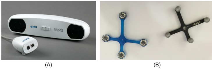
Figure 11.3 (A) Tracking system for active and passive tools; (B) reflecting spheres for passive tracking. Courtesy: NDI.
