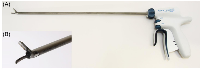
Figure 7.57 Disposable ultrasonic shears. The blade is vibrating against the mobile branch which is covered by synthetics or ceramics (on reusable shears). (A) Completely assembled instrument; (B) Tip: The mobile arm is in an oblique (open) position. From MITI.
