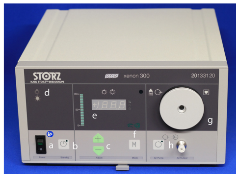
Figure 7.29 Light source: a, main switch; b, standby button; c, light intensity adjustment buttons; d, controls for main/spare light bulb; e, intensity of light; f, manual/automatic light intensity adjustment; g, light cable connector; h, optional air pump switch and connector to reduce fog on telescope lens. From MITI.
