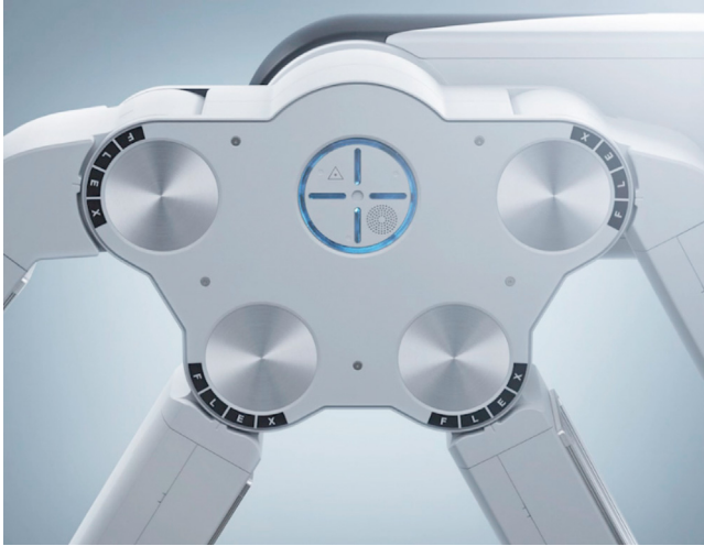
Figure 10.24 A laser targeting system facilitates the optimal positioning of the cart. Once the scope is attached, it has simply to be pointed at the target anatomy and the system will position the boom in an optimized configuration for the procedure. From Intuitive Surgical.
