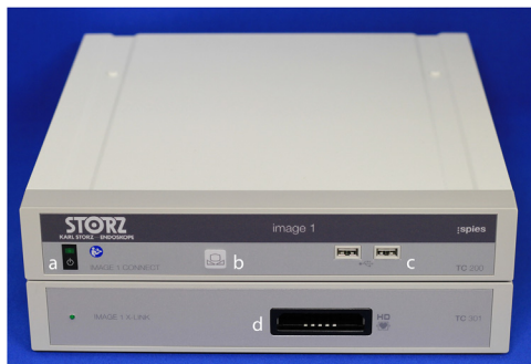
Figure 7.22 Front panel of an image processor (CCU): a, power switch; b, white balancing button; c, USB connectors for mobile storage devices; d, connector for the camera head. From MITI.
