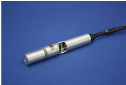
Figure 7.63 Satellite camera: The “internal” camera is able to replace the classical telescope which requires an own trocar. Experimental design with an outer diameter of 10 mm. All from MITI.
