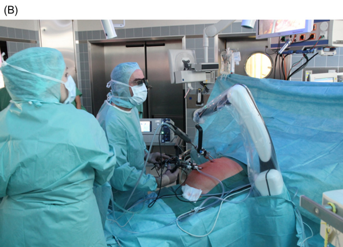
Figure 10.11 (A) The lightweight camera holder SOLOASSIST; (B) the SOLOASSIST in surgery. The universal joint is sterilized. The arm is covered by sterile drapes. All from Aktormed GmbH.
