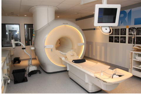
Figure 5.11 Medical MRI scanner: The patient is positioned on the couch (foreground) which will be advanced into the coil. From MITI.
