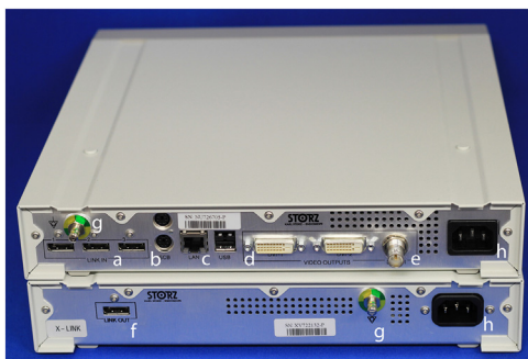
Figure 7.23 Rear panel of the CCU: a, link connectors to other CCUs for image switching; b, SCB (STORZ Communication Bus) connector, bus system to transfer data between other peripheral devices; c, network connector for storage; d, USB connector for portable storage media; e, DVI and composite video outputs; f, link out for video connection to other CCUs; g, electrical ground connector; h, mains plug. From MITI.
