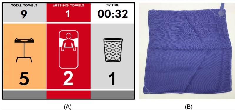
Figure 11.15 (A) Prototype of a surgical RFID application: Counting and localizing of abdominal sponges. In total nine towels are prepared, five are on the Mayo stand, two in the patient, one is used in the bin and one is missing. (B) Surgical sponge with integrated passive RFID tag [25]. All from MITI.
