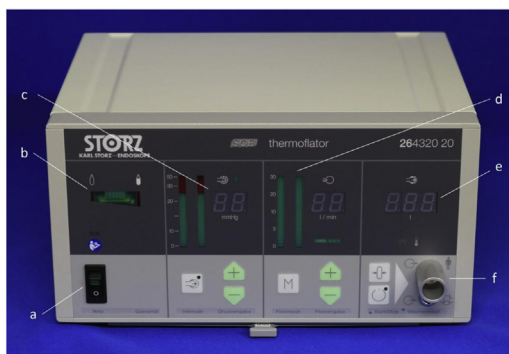
Figure 7.7 Gas insufflator, front panel: a, power switch; b, gas supply; c, intraabdominal pressure; d, insufflation flow; e, insufflated volume; f, tube to patient connector. From MITI.
