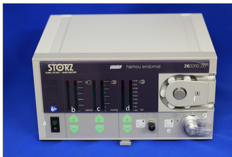
Figure 7.32 Suction/irrigation device: a, main switch; b, maximum flow adjustment and display; c, maximum pressure adjustment; d, minimum aspiration vacuum adjustment and display; e, standby button; f, instillation tube notch; g, aspiration tube connection. From MITI.
