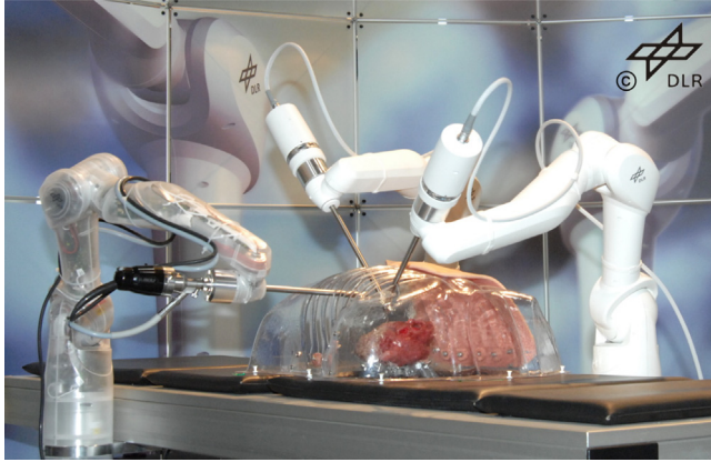
Figure 10.35 MiroSurge telemanipulator: Three MIRO robots mounted on an operating table. White MIROs carrying MICA instruments with force/torque sensing, transparent MIRA carrying a stereo endoscope. From Tobergte A, Passig G, Kuebler B, Seibold U, Hagn UA, Fröhlich FA, et al. MiroSurge—advanced user interaction modalities in minimally invasive robotic surgery. Presence 2010;19(5):400–14 [36].
