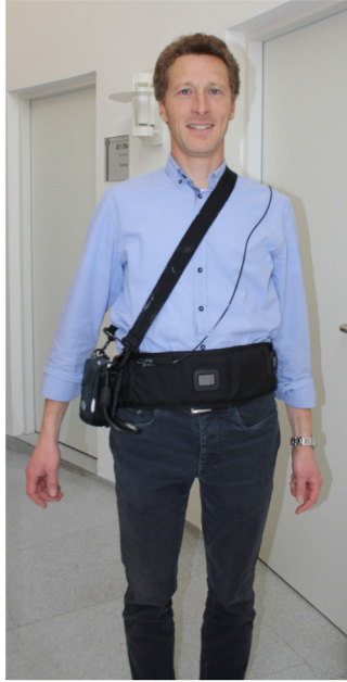
Figure 5.58 Capsule endoscope image receiving box. From MITI.
