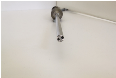
Figure 7.25 Full-HD stereo telescope with fixed camera head and four light emersion points with the possibility to switch to 2D by using only one imaging channel. From MITI.
