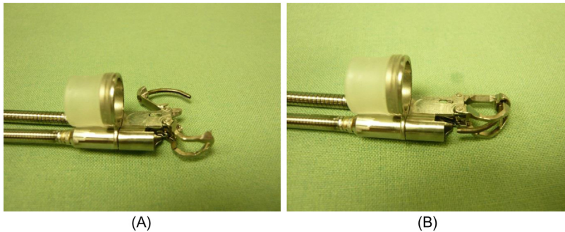
Figure 9.22 First prototype of the endoscopic sewing machine: (A) Starting position; (B) closed. All from MITI.
