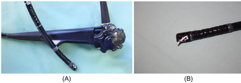
Figure 8.3 (A) The handling of a duodenoscope with the Albarran lever; (B) tip of the instrument with the lever for angulation. All from MITI.
