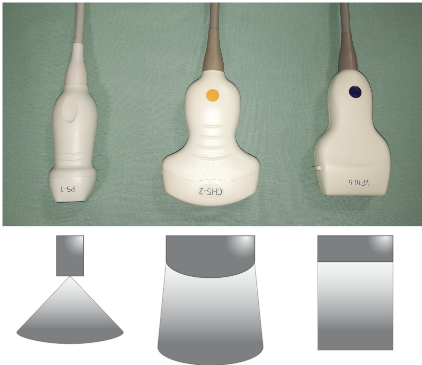
Figure 5.18 A selection of typical transducers. Left: Sector scanner, most often used in cardiology; middle: convex scanner, standard in abdominal US; right: linear scanner. In addition, a large number of purpose-designed probes (transanal, transvaginal, transesophageal, etc.) are available. Courtesy: PD Dr. M. Kranzfelder, Klinikum rechts der Isar.
