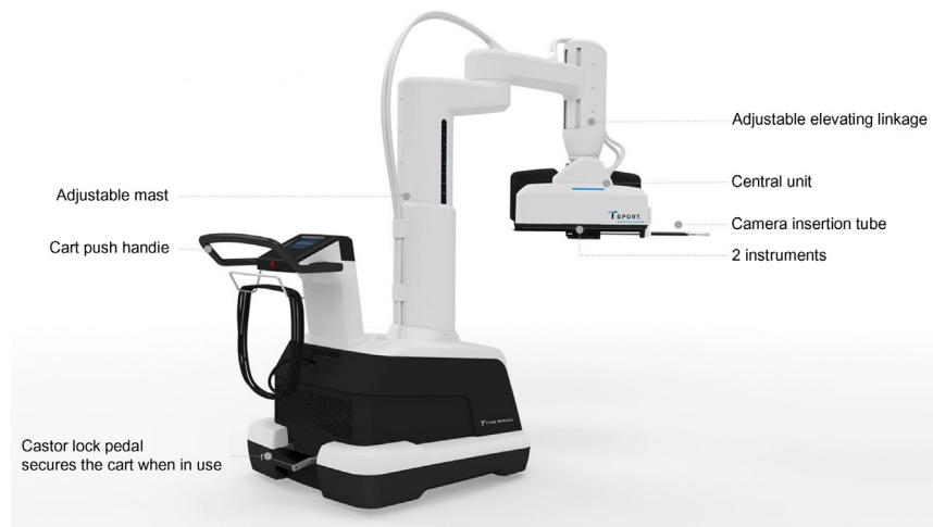
Figure 10.29 Patient Cart and CIT in the working configuration for transportation, the boom can be lowered and folded into a very compact configuration. From Titan Medical, Inc.
