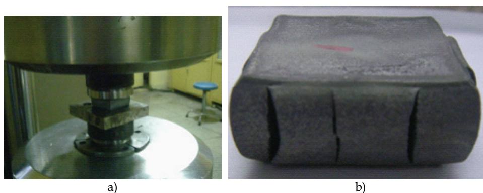
Fig. 29. The experiment to determined the compressing stress of the shielding materials' sample. a) The compressing stress test of the sample, b) The compressing stress sample of Jxa1 when it was compressed to 50%
