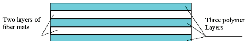
Fig. 12. Sandwich structure of PLA and fibril composites for compressive molding
