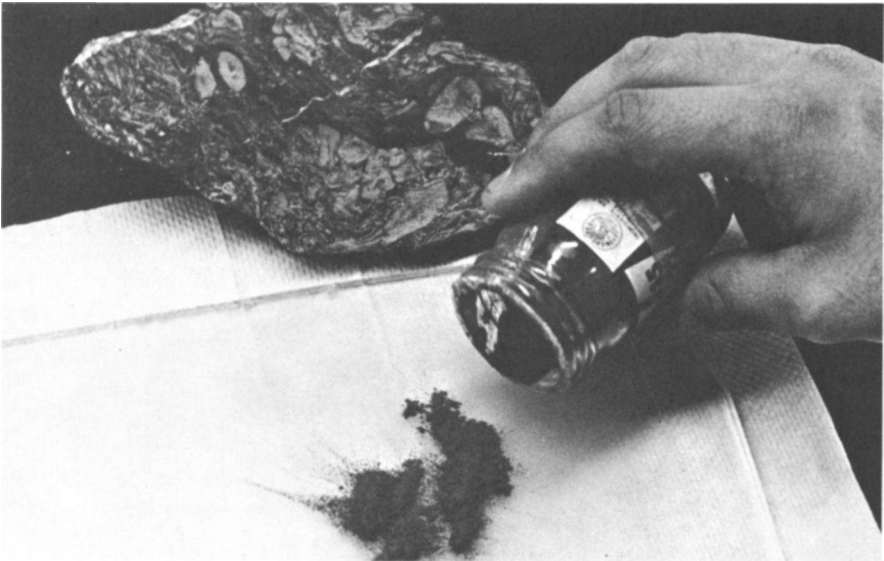
Making a coal-ball peel. Step 1: After the coal ball has been sawed, it must be ground perfectly flat. A small amount of number 400 silicon carbide grit is used on a sheet of plate glass.
