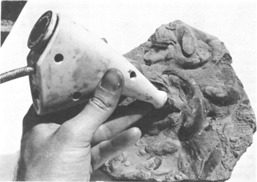
Vibrating tools are useful to remove matrix rapidly from such specimens as these fossil clams.
