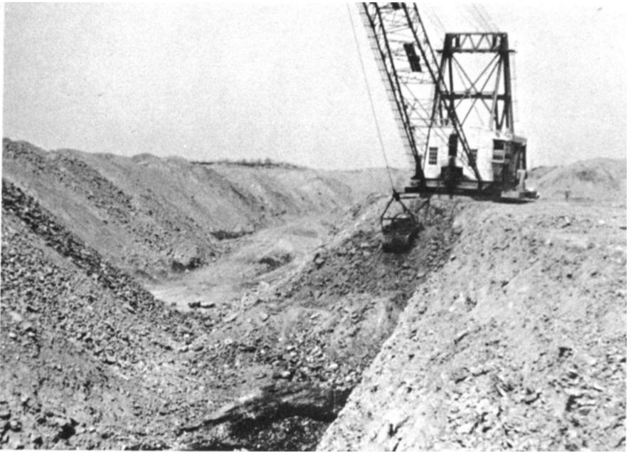
Coal strip mine in action. Big dragline scoops up the gray shale overlying the coal and piles it to one side. Dugger, Indiana.
