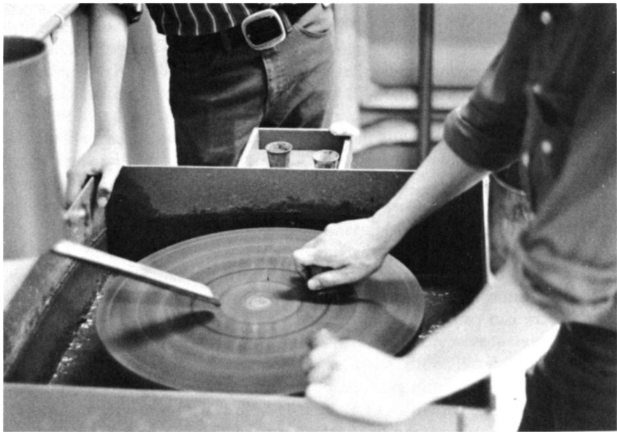
Cast-iron flat lap grinds flat sections for microscope examination or for preparing coal balls or petrified wood.
