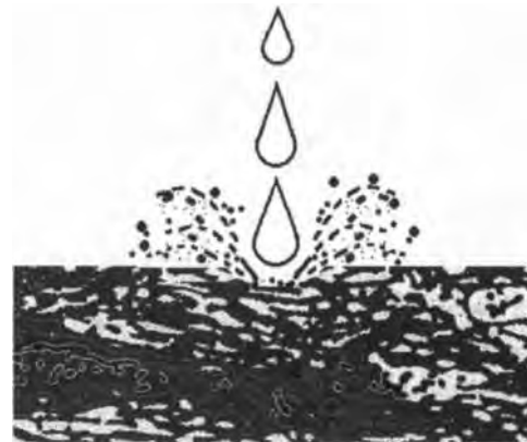
Fig.S.21: Raindrops cause splashing of soil particles and may lead to soil erosion.
