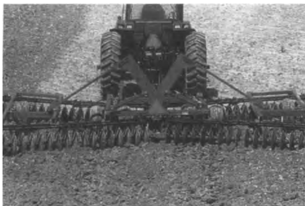
Fig.H.1: A tractor-mounted disc harrow.
