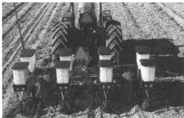
Fig.C.37: Tractor-mounted combined seed and fertilizer drill for contact placement of fertilizer.
