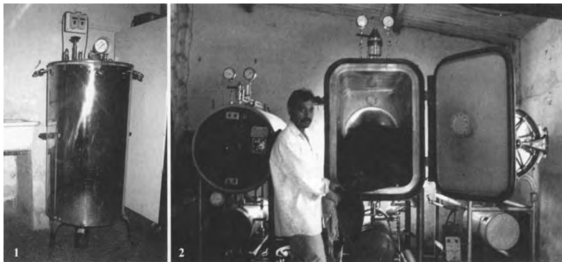
Fig.A.42: Types of autoclave. 1. Vertical type, 2. horizontal type.
