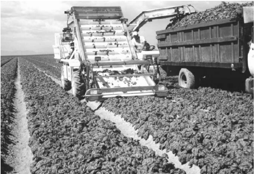
Fig. 6. Band saw harvester cutting fresh market spinach.
