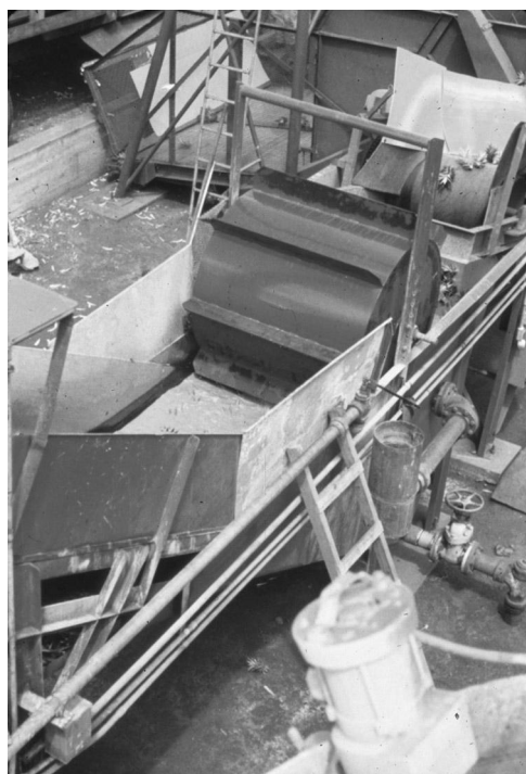
Fig. 9.13. Pineapple dipping equipment for treating seed materials with fungicides for butt-rot control or insecticides to control scale or mealybugs.
