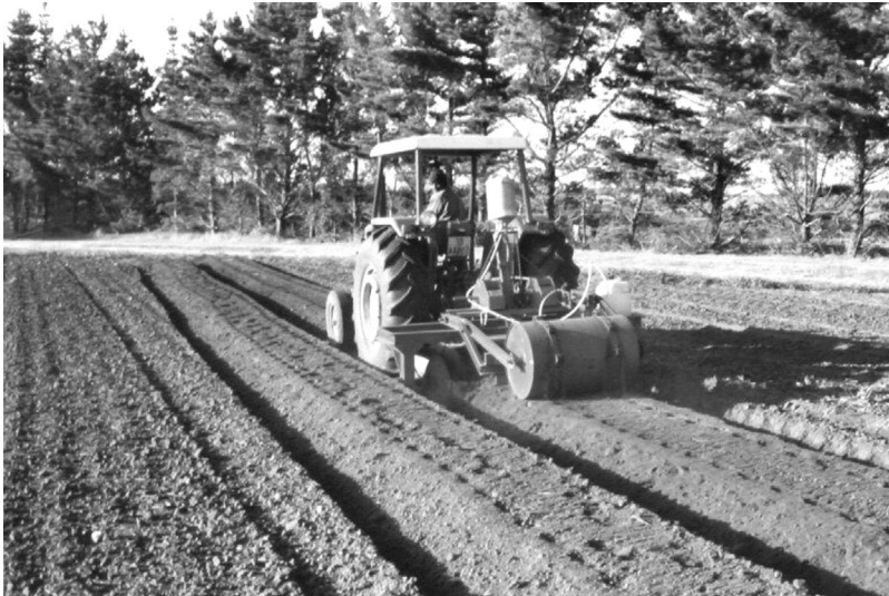
Fig. 6.3. Ridger used in South Africa to facilitate drainage in heavy soils. Protrusions on the roller establish the plant spacing. (Photo courtesy of Graham Petty.)
