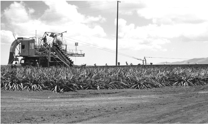
Fig. 6.21. Bin-mounted ‘parasitic’ harvester that moves with the truck while fruit are being picked.
