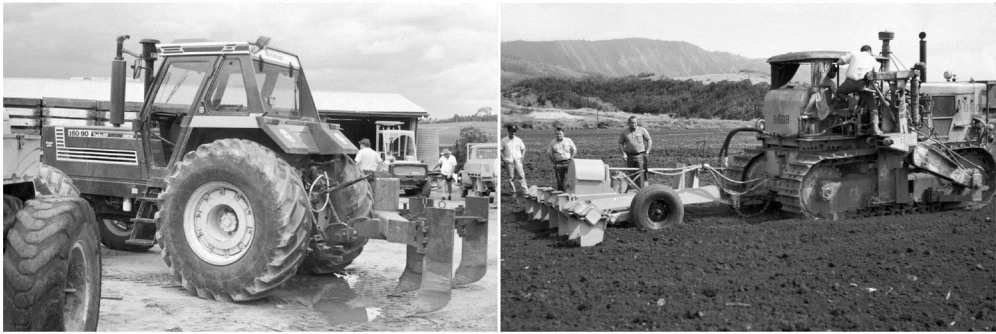
Fig. 6.2. Subsoilers used in Queensland, Australia, and in Hawaii, to improve soil drainage (photos courtesy of D. Bartholomew (left) and K.G. Rohrbach (right)).
