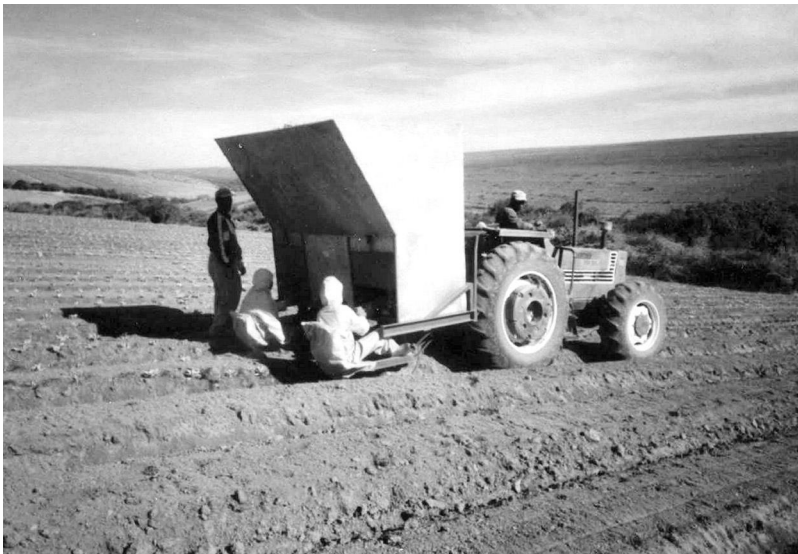
Fig. 6.14. A relatively simple pineapple planter used on a pineapple farm in South Africa (photo courtesy of Graham Petty).
