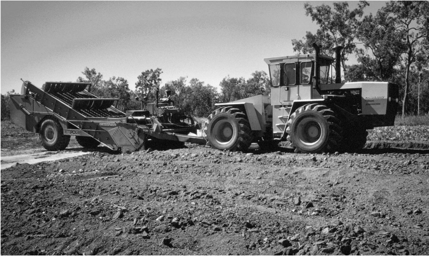
Fig. 6.4. Rock picker used in northern Queensland, Australia, to remove large rocks from pineapple fields prior to planting (photo of Duane Bartholomew).
