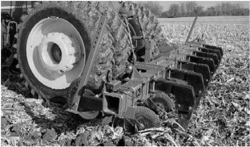
FIGURE 11.1. Subsoiler equipped with coulters opens compact soils while leaving much of the residue on the surface. (Photo courtesy of Adrian Puig, Everglades Farm Equipment, Belle Glade, Florida, and Matthew A. Weinheimer, John Deere Des Moines Works.)
