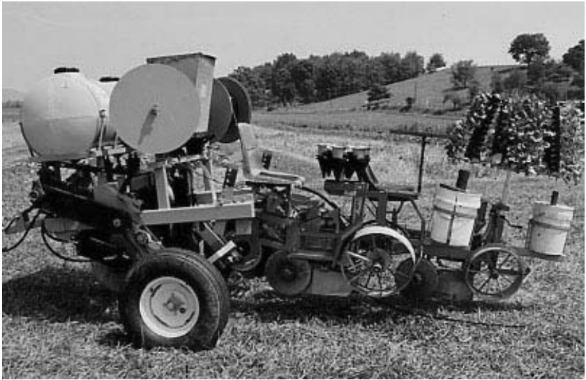
FIGURE 10.7. Subsurface Tiller Transplanter developed by Dr. R. D. Morse and associates at Virginia Polytechnic Institute and State University, Blacksburg, Virginia. The transplanter is capable of loosening compact soil in a small band (2.5-4 in wide \times 6-10 in deep), setting transplants in heavy residues, firming loosened soil around plants, applying needed fertilizers and pesticides, and laying drip irrigation tubing. (Photo courtesy of Dr. R. D. Morse.)
