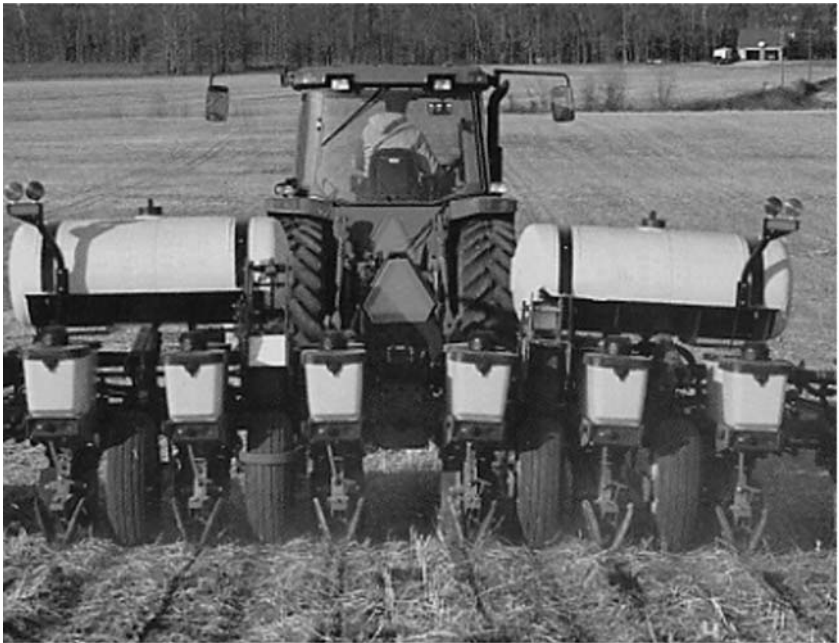
FIGURE 10.3. Seeder capable of planting seeds and applying liquid fertilizer in 8 or 12 rows of residue mulch in varying terrain. (Photo courtesy of Adrian Puig, Everglades Farm Equipment, Belle Glade, Florida, and Matthew A. Weinheimer, John Deere Des Moines Works.)
