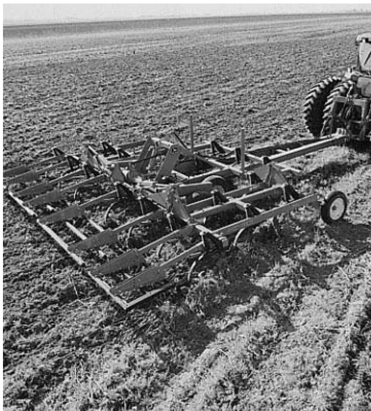
FIGURE 10.6. Multiple chisel plow as a unit opens soil, leaving considerable residue on surface. The unit is designed to stay level, keeping sweeps or shovels at uniform depth. (Photo courtesy of Adrian Puig, Everglades Farm Equipment, Belle Glade, Florida, and Matthew A. Weinheimer, John Deere Des Moines Works.)
