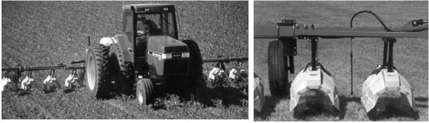
FIGURE 11.3. Hooded sprayer. Spraying inside a hood over primary crop row (left) permits spraying it with fungicides or insecticides with little or no injury to beneficials on cover crops in aisles. By centering the spray nozzle between the hoods (right), herbicide application can be directed to the cover crops in aisles to suppress or terminate it without damage to the primary crop which is protected by the hoods. (Photos courtesy of Steve Clausen, Redball, LLC, Benson, Minnesota.)
