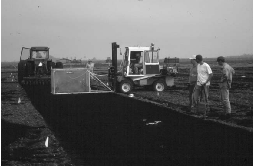
FIGURE 2.2. A device for measuring \text{CO}_2 within a plastic chamber is being lowered over freshly tilled soil to document the effect of tillage on microbial activity and resultant \text{CO}_2 evolution. (Photo courtesy of Dr. Don Reicosky, USDA.)
