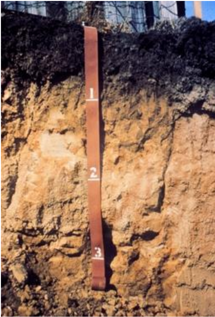
Photo 9. —A soil with an ochric epipedon about 15 cm thick. The dark colored ochric epipedon is too thin to be a mollic or umbric epipedon.
