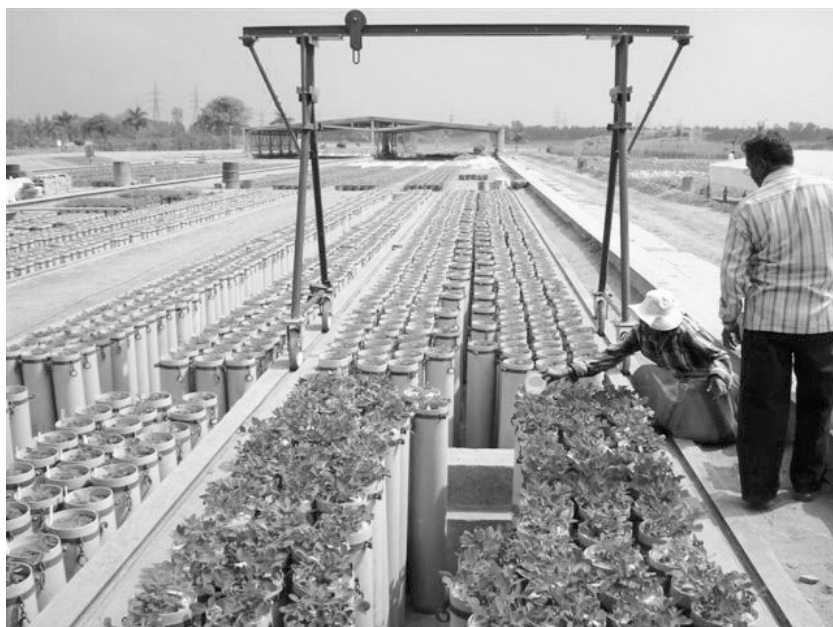
Fig. 8.6. Characterization of the variation in transpiration across growing time of the reference collection of groundnut germplasm using a mini-lysimetric system.
