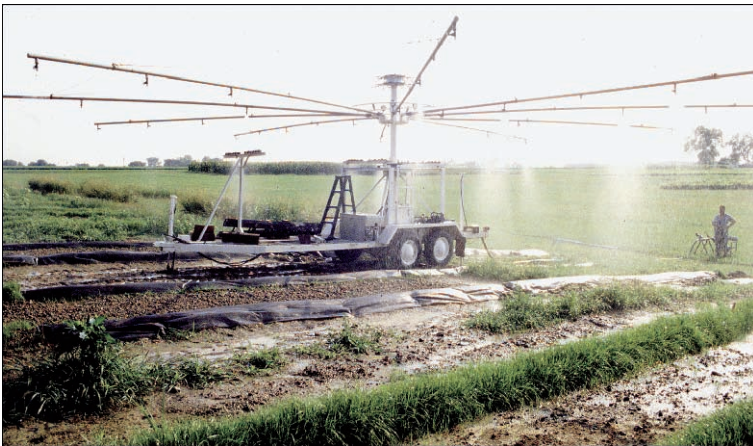
Plate 9 The Swanson type rotating boom rainfall simulator (Photo by H. Blanco). The simulator booms are equipped with nozzles positioned at radii of 1.5, 3.0, 4.5, 6.0, and 7.6 m. Booms and nozzles rotate in a circle, and the wetted diameter is about 16 m
