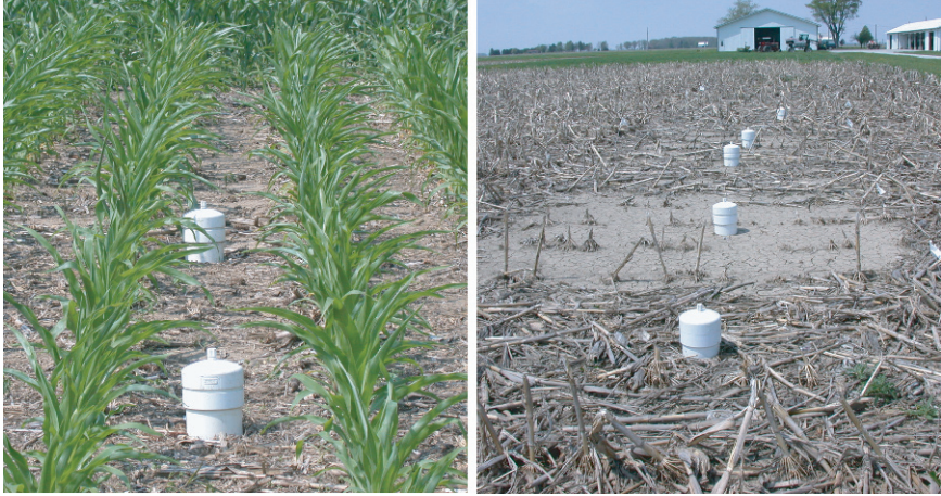
Plate 67 The closed chamber method consists of a gas sampling chamber made of PVC with a bottom section (30 cm long \times 15 cm diameter) inserted into the ground, and a lid equipped with a gas sampling port (Photo by H. Blanco). Air samples withdrawn from the chamber are stored in evacuated vials for the soil gas (e.g., CO 2 , CH 4 ) analyses
