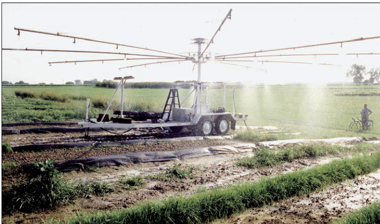
Fig. 2.6 The Swanson type rotating boom rainfall simulator (Photo by H. Blanco). The simulator booms are equipped with nozzles positioned at radii of 1.5, 3.0, 4.5, 6.0, and 7.6 m. Booms and nozzles rotate in a circle, and the wetted diameter is about 16 m
