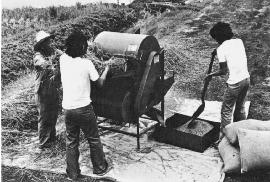
Figure 13.5 IRRI-designed, portable axial-flow threshers are now being used by farmers in India, Sri Lanka, Thailand, and the Philippines.
