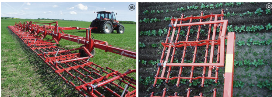
Fig. 17.1 Whole crop cultivation in cereals with a 27 m wide spring-tine harrow (a), harrowing in faba beans (b). Photos Einböck, Agritechnika 2005
