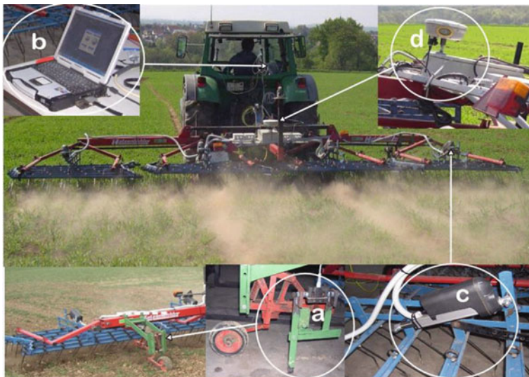
Fig. 17.3 Prototype of an automatically controlled flexible tine harrow containing soil sensor (a), computing control unit (b), motor to change the tine angle (c), and RTK-DGPS for positioning (d)
