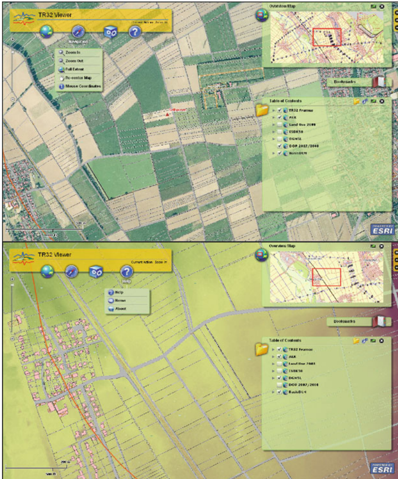
Fig. 13.7 WebGIS interface of the TR32 project: aerial imagery (DOP), cadastral land parcel map with building features (ALK), and ATKIS ( top ); official elevation model from airborne LIDAR campaigns (DEM5L) and ALK ( bottom ) ( http://www.tr32db.de )
