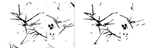
Fig. 8.5 Binarisation and preprocessing of the difference image in Fig. 8.4. Left : the result of the thresholding, right : the result after applying morphological operators (closing with circle of 5 pixel diameter) and area size selection (regions with more than 30 pixel), as well as discarding regions which are cut by the image border. Foreground objects are black, the background is white
