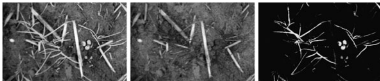
Fig. 8.4 Example for the difference ( right ) of an infrared ( left ) and red ( middle ) image. Plants are bright due to the spectral difference in the red and infrared, background objects like dead material (mulch, stones) disappear in the difference image. Gray values were stretched to increase the contrast for the print version
