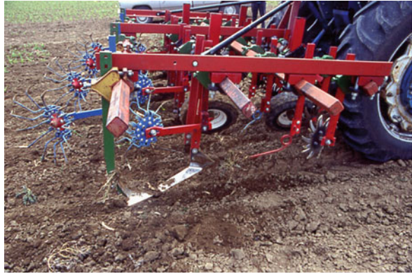
Fig. 17.5 Bezzerrides-cultivator for in-row and intra-row weed control in maize
