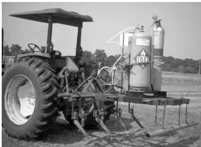
Fig. 10.10. Application equipment for soil injection of 1,3-D soil fumigant by chisel injection. Six chisels are arranged on the tool bar, each spaced 30 cm apart. The cylinder of 1,3-D is pressurized by nitrogen gas. (Photo: D.W. Dickson.)
