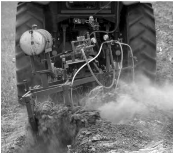
Fig. 10.9. Plough-down application of the soil fumigant 1,3-D. (Photo: D.W. Dickson.)
