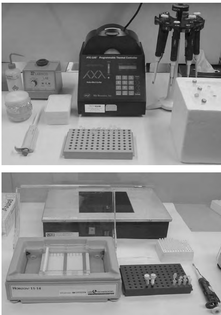
Fig. 3.6. Equipment required for PCR (top), electrophoresis and visualization of the PCR product on agarose gel (bottom).
