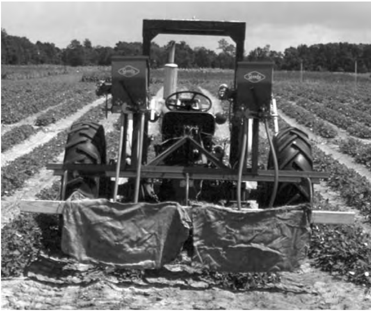
Fig. 10.11. Application equipment for a post-plant application (peg initiation) of a non-fumigant nematicide. The granular nematicide is spread in rows over vines by a 14 inch wide row bander. The burlap bags knock the granules off vines to the soil surface. (Photo: D.W. Dickson.)
