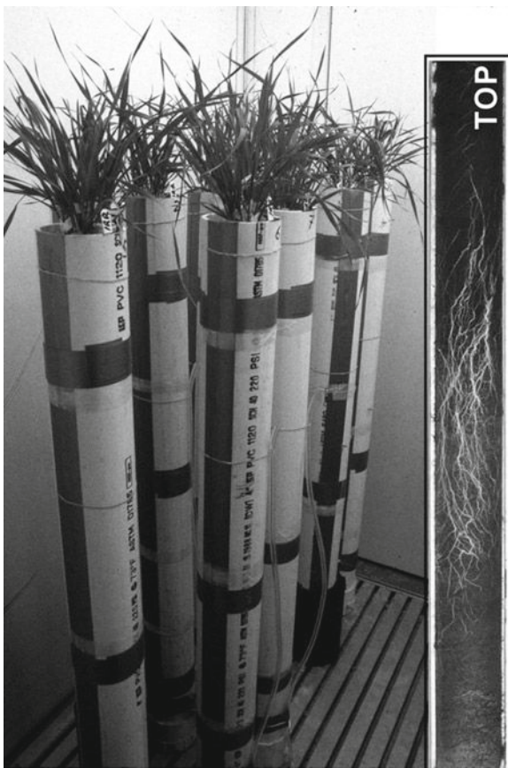
Fig. 4.15 Split PVC tubes with growing wheat plants; the inset on right presents the exposed soil core with some of the roots on the surface
