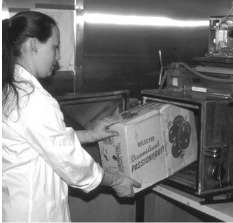
Fig. 6.2. Small-scale research fumigation of test fruit. Potential differences in efficacy and commodity quality between small, research-scale and large, commercial-scale treatments must be addressed before phytosanitary treatments can be offered to industry. (Photograph by R. Corcoran)
