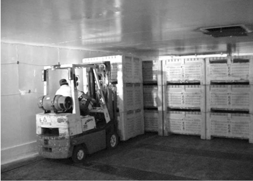
Fig. 10.1. Fruit being prepared for fumigation with methyl bromide in a sealable purpose-built chamber.
