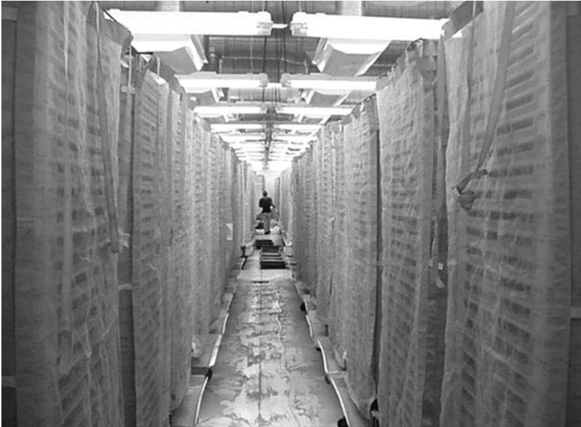
Fig. 5.2. Mass rearing of Mediterranean fruit fly in Guatemala for production of insects for sterile release programmes against the pest worldwide. Capacity is for 3.5 \times 10^9 flies/week; half that is currently being produced. Shown are towers of trays holding larvae in artificial diet as a rearing medium, held in a large controlled environment room.
