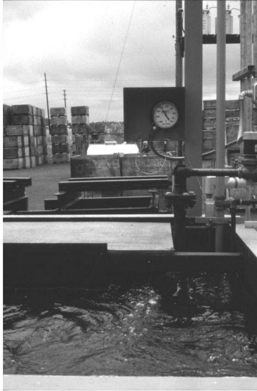
Fig 8.5. A hot-water treatment unit for disinfesting fruit in palletized batches. Note the active circulation of the water.
