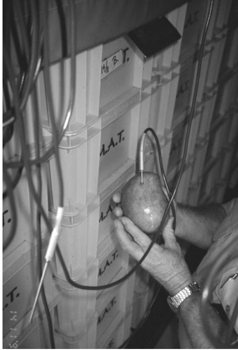
Fig. 8.4. Resistance temperature detector probes used to control and monitor fruit treatment in a forced-air heating unit. The probe monitoring fruit pulp temperature would be one of several distributed throughout the load, each inserted into the largest fruit of the plastic basket. (Photograph by R. Jordan)
