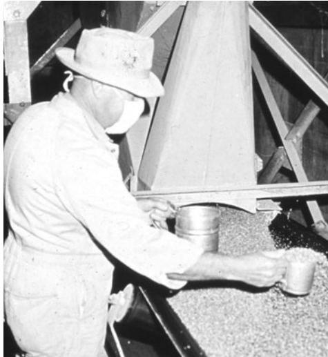
Fig. 5.6. Sampling a grain stream for insect infestation. The sample will be sieved to separate insects from the grain. Internal stages cannot be determined. Automated sampling is a feature of some modern terminals but pest identification should be done by inspectors. (Photograph by M. Bengston)
