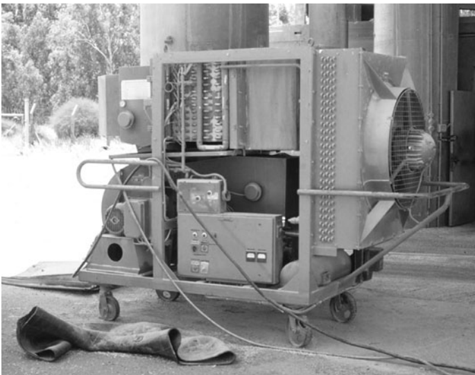
Fig. 7.2. A mobile refrigerated aeration unit suitable for small bin lots such as seeds.
