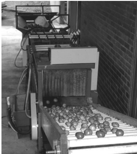
Fig. 12.1. A re-circulatory pesticide spray treatment module of a tomato packing line. The spray bars are seen on the top centre of the unit, the further set high pressure low volume and the nearer set high volume low pressure; the tank of insecticide can be seen under the unit. Application rates are controlled by pesticide concentration, nozzle aperture and conveyor speed.
