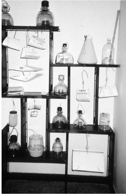
Fig. 5.4. A range of designs of fly trap. Being able to adequately sample feral populations of quarantine pests is fundamental to the design and proper functioning of phytosanitary systems. Trap structure, colour, bait and placement may all affect capture.
