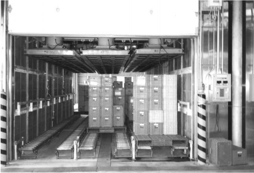
Fig. 8.2. Inside a forced-hot-air facility similar to that in Fig. 8.1 showing fans for the circulation of air down through carriers with perforated bottoms. Entry is from the far side and egress from the open side to a secure packing area.
