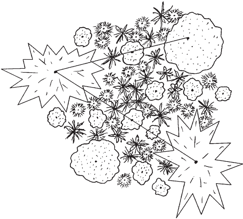
FIGURE 11.1. A disarrayed midpoint design, in which plants are located midway between two taller species.
