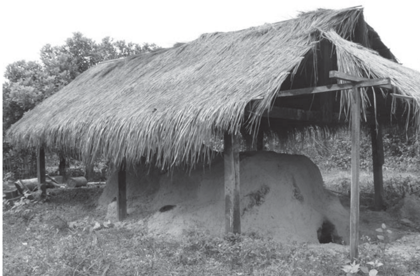
Fig. 1.1. Primitive method of charcoal production in Ratnakiri, Cambodia.
