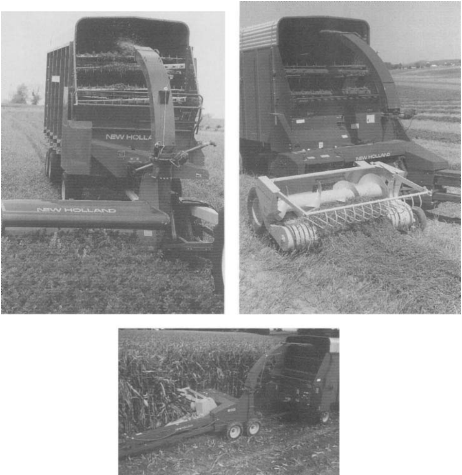
FIGURE 15.10 Forage choppers have contrasting heads, depending on the type of forage to be chopped. ( Top left ) Direct-chop head. ( Top right ) Swath pickup head. ( Bottom ) Corn head. (Courtesy of New Holland North America, Inc.)
