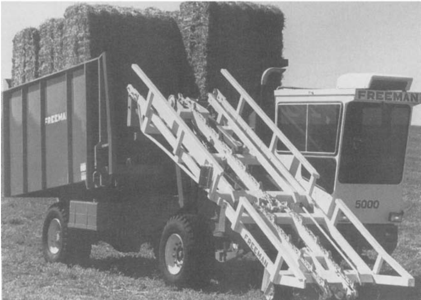
FIGURE 15.9 (Top) Bale wagon for handling small rectangular bales. (Courtesy of New Holland North America, Inc.) (Bottom) Bale wagon for handling large rectangular bales. (Courtesy of J. A. Freeman & Son, Inc.)
