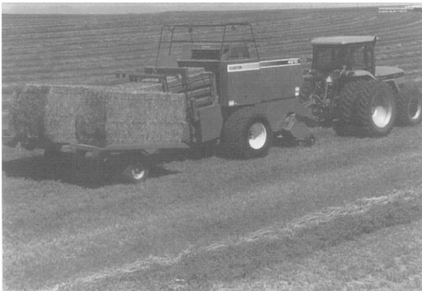
FIGURE 15.7 Large rectangular baler with a bale accumulator. (Courtesy of AGCO Corporation.)
