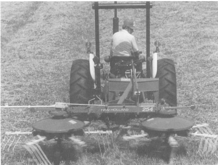
FIGURE 15.4 A tedder is commonly used to turn grass-hay windrows to enhance drying. (Courtesy of New Holland North America, Inc.)
