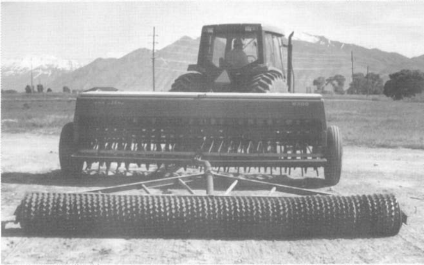
FIGURE 9.3 Seeding small-seeded forage legumes and grasses with a drill is successful if the seed is covered after it falls to the ground. Methods of covering include drag chains, following the seeding operation with a roller compactor (above), or press wheels that push the seed into the ground immediately behind the drill. Drag chains by themselves are the least effective, but when used in conjunction with a roller compactor, excellent results may be obtained. (Photo by author.)
