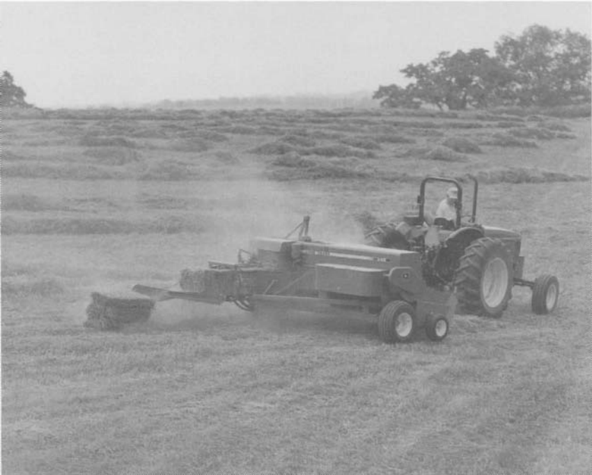
FIGURE 15.6 Progression of baler technology. ( Top ) An early John Deere Power Press stationary baler. ( Bottom ) A pull-type baler which makes small-rectangular bales. (Courtesy of Deere and Company.)
