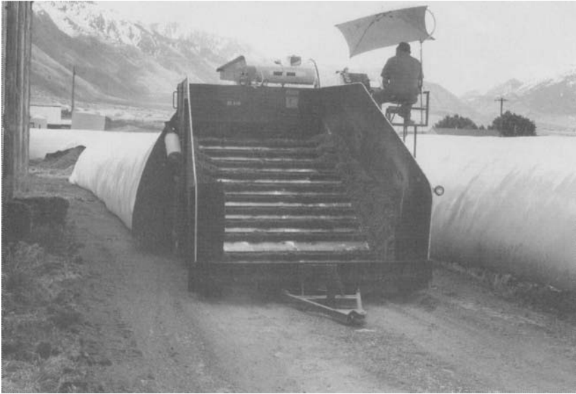
FIGURE 15.13 Bagging unit for placing silage in long plastic bags. (Photo taken by author.)
