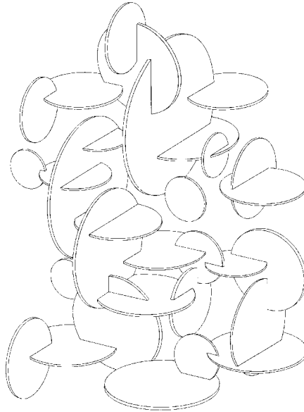
FIGURE 17.25 Three-dimensional conceptual model of disc-shaped fractures which are of random size and oriented orthogonally. (From Long, J. C. S., Gilmour, P., and Witherspoon, P. A. 1985. A model for steady fluid flow in random three-dimensional networks of disc-shaped fractures. Water Resour. Res. 21(8):1105-1115. With permission.)
