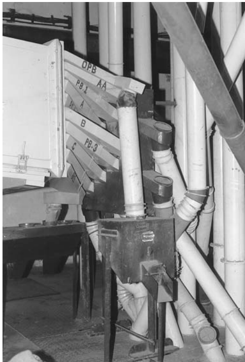
Fig. 10 Grading of coffee beans. (Courtesy of Chamundi Coffee Curing Works, Mysore, India.)
