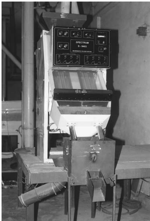
Fig. 12 Electronic color sorter (Sortex). (Courtesy of Chamundi Coffee Curing Works, Mysore, India.)
