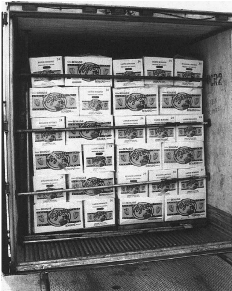
Fig. 2 Bracing systems used to prevent produce from shifting backward to the rear doors.
