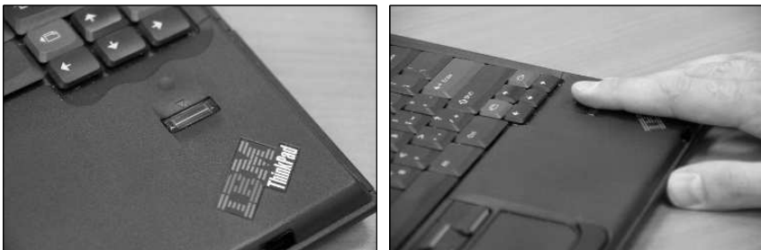
Fig. 23.1. A swipe fingerprint reader is embedded into an IBM notebook to prevent anyone other than the owner from accessing data on it.
