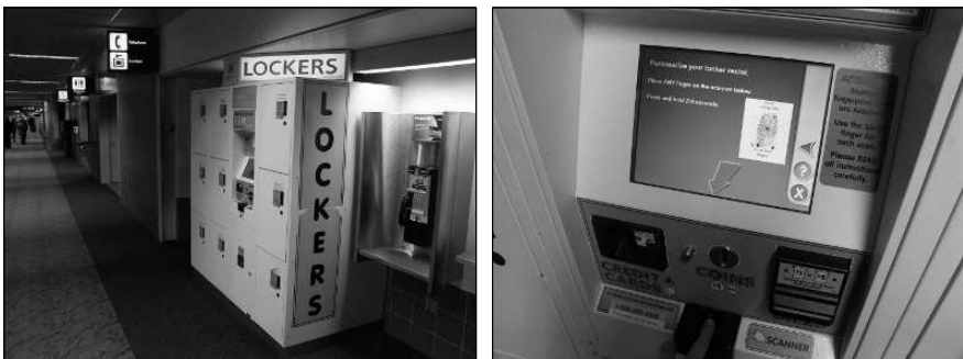
Fig. 23.2. Rental lockers at an Airport. These lockers, manufactured by Smarte Carte, use biometrics for locker access control.
