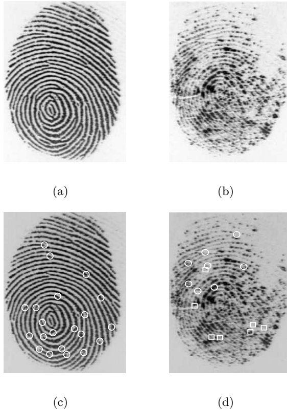
Fig. 17.1. Minutiae extraction results for fingerprint images of varying quality. (a) A good quality fingerprint image. (b) A noisy fingerprint image. (c) Minutia points detected in the good quality fingerprint image by an automatic minutiae extraction algorithm. (d) Minutia points detected in the noisy fingerprint image. The circles represent true minutia points while the squares represent false (spurious) minutiae. While no spurious minutia is detected in the good quality fingerprint image, several false minutia points are detected when the fingerprint image quality is poor.
