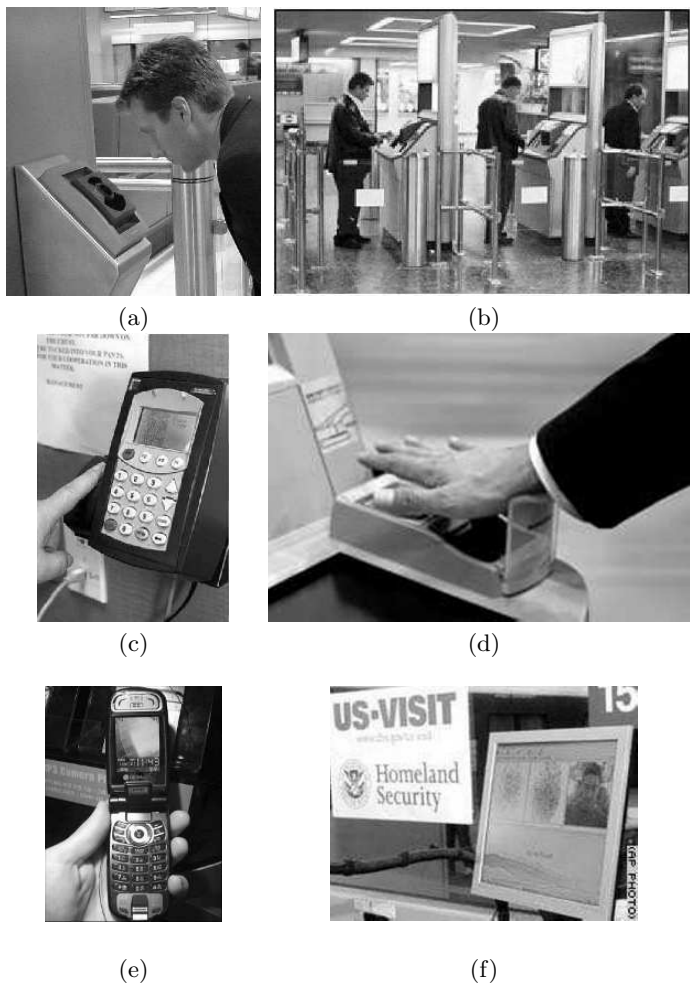
Fig. 1.5. Biometric systems are being deployed in various applications. (a) The Schiphol Privium program at the Amsterdam airport uses iris scans to validate the identity of a traveler ( www.c1.cam.ac.uk ). (b) The Ben Gurion airport in Tel Aviv uses Express Card entry kiosks fitted with hand geometry systems for security and immigration ( www.airportnet.org ). (c) A few Kroger stores in Texas use fingerprint verification systems that enable customers to render payment at the check-out counter. ( www.detnews.com ). (d) Contactless palm-vein systems have been installed in some ATMs in Japan ( www.fujitsu.com ). (e) A cell-phone that validates authorized users using fingerprints and allows them access to functionalities such as mobile-banking ( www.mobileburn.com ). (f) The US-VISIT program currently employs two-print information to validate the travel documents of visitors to the United States ( www.dhs.gov ).
