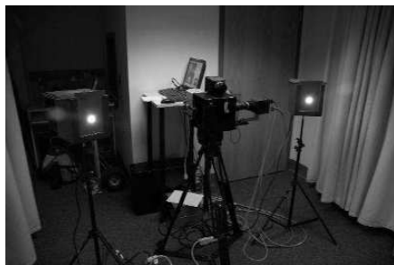
Fig. 15.7. Camera and lighting setup for image collection
