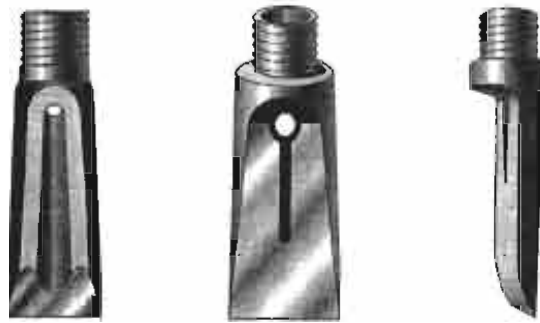
Figure 5.2.7. Various designs of jetting drill bits.
