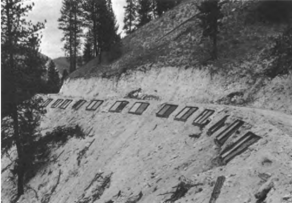
Fig. 70. Research on the protective effect of surface mulching. A series of small experimental plots are used: measurements of runoff and silt are not made (Idaho, USA). (By courtesy of U.S. Forest Service.)
