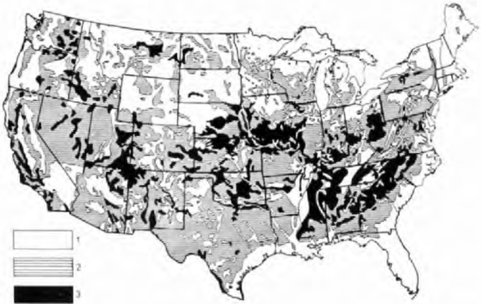
Fig. 186. General map of the distribution of erosion on cultivated soil in the USA. A – slight or none, B – moderate – 25 to 75% of topsoil lost, may have some gullies, C – severe – more than 75% of topsoil lost, may have numerous or deep gullies. Includes severe geological erosion in parts of low rainfall area. Many small areas could not be shown at this scale.
