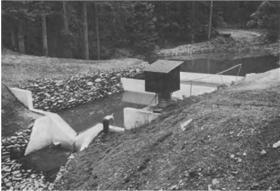
Fig. 77. Measurement of water runoff and silt sedimentation on an experimental plot. (By courtesy of U. S. Forest Service.)
