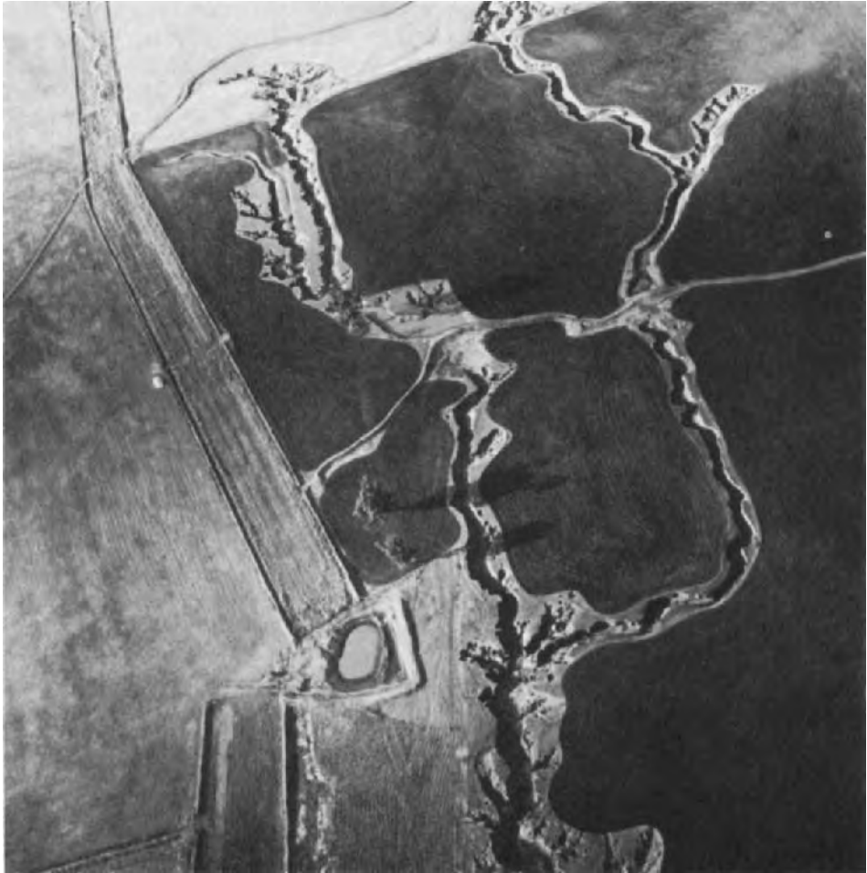
Fig. 182. Comprehensive measures taken against sheet and gully erosion, including contoured banks, grassed water verges and dams. The picture also shows gully growth owing to tunnel erosion (northern Victoria). (By courtesy of Soil Conservation Authority, A.S.)
