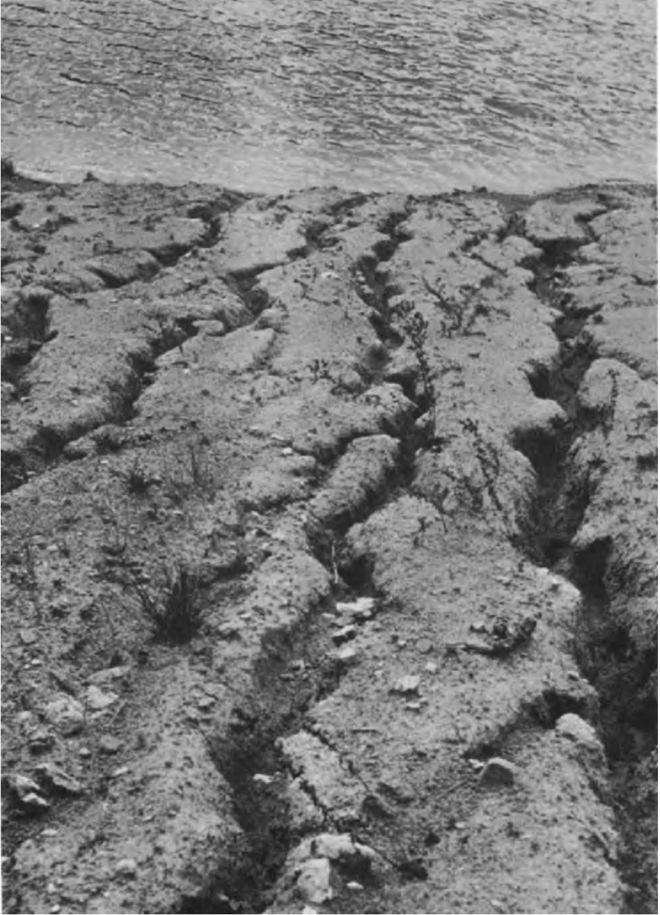
Fig. 100. Rills formed on unprotected, bare soil of low permeability on moderate gradient (Hriňová dam, Czechoslovakia). (Photo D. Zachar.)
