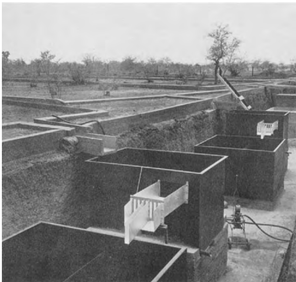
Fig. 68. A well-equipped erosion control research station with a series of suitably large elementary plots with reduction vessels (Quahiquoya, Upper Volta). (The author's collection of photographs.)
