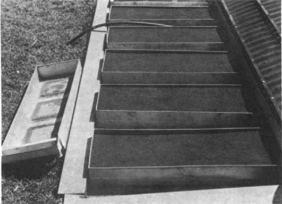
Fig. 72. Soil trays for measuring splash and wash erosion. The porous tiles in the false floor can be seen in the empty tray on the left. (Photo N. W. Hudson.)
