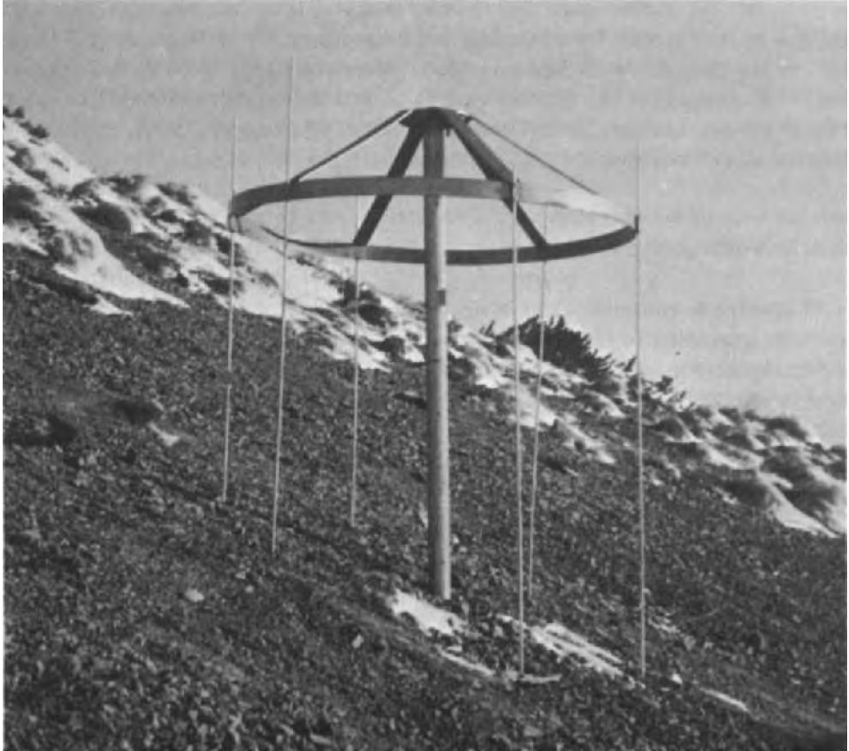
Fig. 66. Another method of measuring surface changes caused by erosion, deposition, frost, or other processes by means of a motionmeter. a – general view, b – aluminium plate – detail (Belanské Tatry Mountains, Czechoslovakia). (Photo R. Midriak.)
