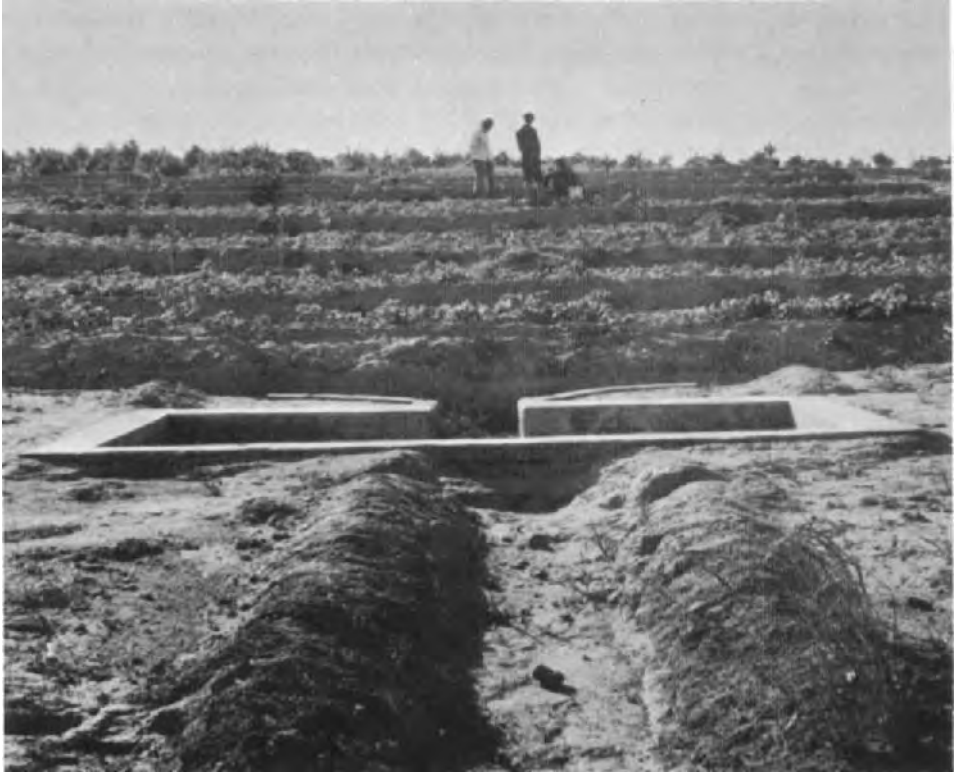
Fig. 67. View of a stationary runoff plot with a simple retention trough in use on an erosion control research station in China. (The author's collection of photographs.)
