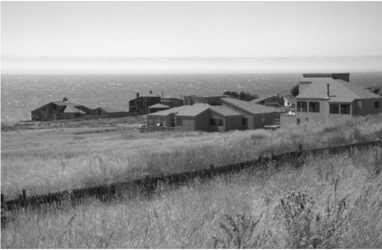
Figure 13.1 Fitting buildings to the landscape. Buildings at Sea Ranch, on the Northern California coast, are designed to blend into the landscape. Fences and decorative landscaping are not allowed.
