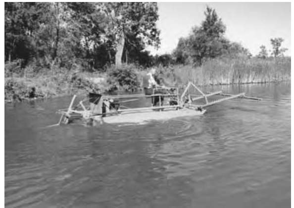
The Hockney Weed Cutter is a self-propelled underwater weed cutter with a proven track record.
