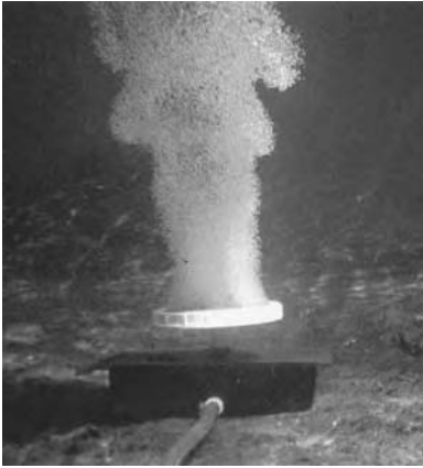
An air line connects to the aeration head, which produces bubbles that lift bottom water to the surface. (From Vertex Water Features, Deerfield Beach, FL.)
