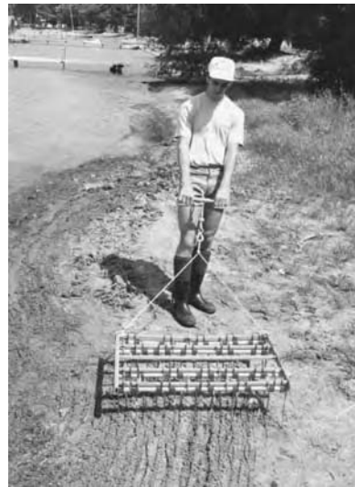
The teeth are staggered from row to row so there is only about an inch between teeth when the rig is dragged.
