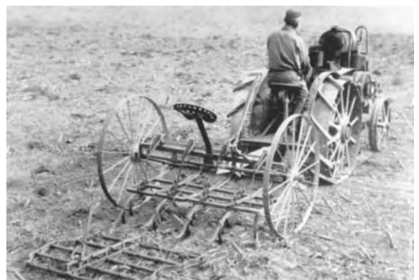
A spike tooth drag and a spring tooth harrow working in a wheat field in 1917. (From Budd, T., Farming Comes of Age , Farm Progress Companies, Inc., Carol Stream, IL, 1995. With permission.)
