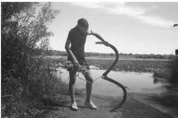
The "three-wedge" drag can be made from a rebar or from plate steel. This one has been cut from plate steel. It is 4 feet long overall. The inside radius of the curve is 12 inches. If made from rebar, start with a bar 7 feet long and then bend it. This is a good drag to use for milfoil because it brings the plants in.
