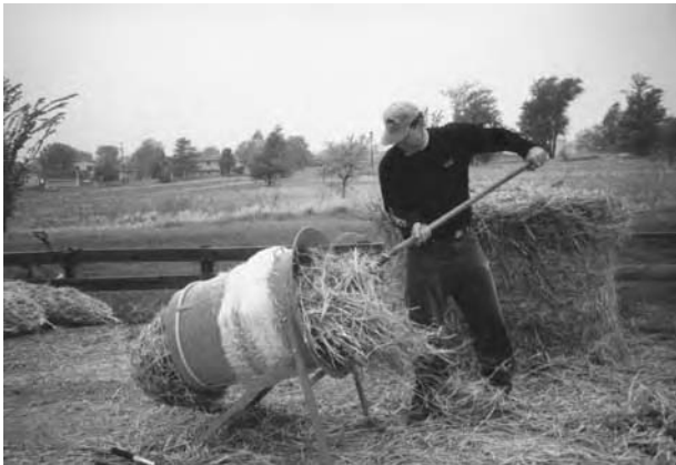
At this site, barley was delivered in 600-pound bales. Barley straw is inserted into the Christmas tree bailer, which feeds out a mesh bag as the straw is pushed through.
