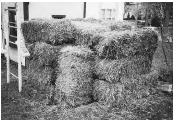
Conventional barley straw bales weigh about 40 pounds and the straw is tightly packed.
