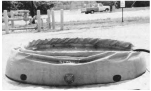
The sides rise as dredge discharge water levels rise. Both types of tanks are made by the Fol-Da-Tank Company (Rock Island, Illinois).
