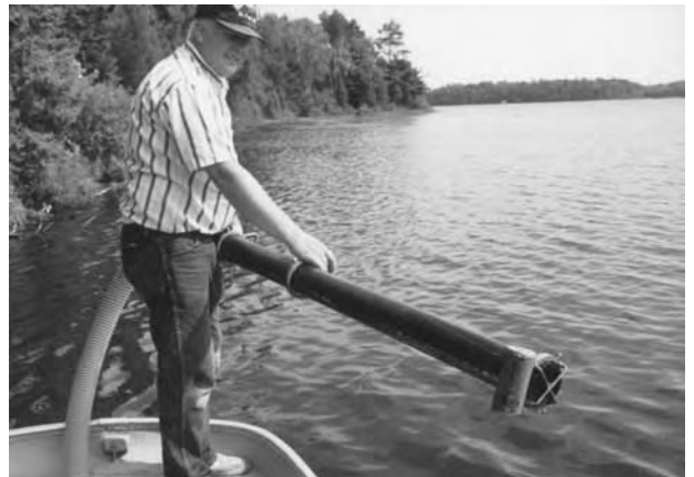
This suction intake is a piece of 3-inch plastic pipe with a steel wire guard over the intake to keep out 1.5-inch rocks that could plug the pump. The bar on the bottom keeps the intake about an inch off the bottom. Handles are attached using hose clamps.
