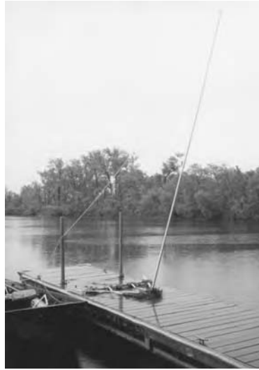
The boat-towed bottom cutter is 6-feet wide and has a 15-foot telescoping handle. When a tow rope is tied to the handle, it pivots at the cutter connection, leaving the cutter on the bottom.
