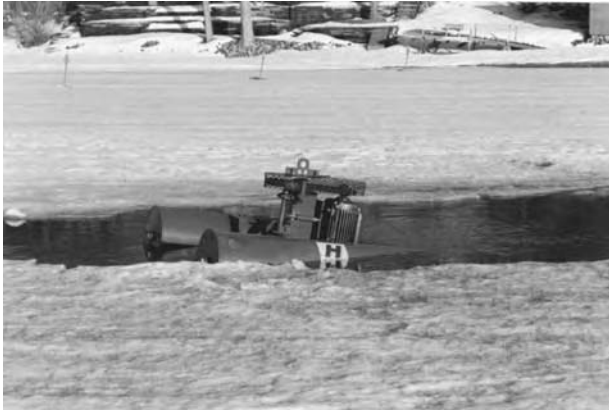
Another style of pump-and baffle-system uses an intake mounted on a floating platform. The hydraulic pump delivers low oxygenated lake water to the baffle component.
