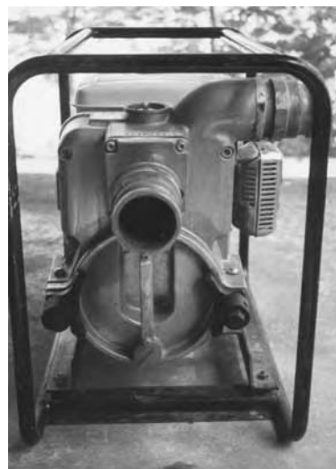
Centrifugal pumps are commonly used at construction sites for dewatering. They are not commonly used to pump lake sediments, but they can.
