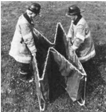
Two people can set up a tank in 30 seconds.
