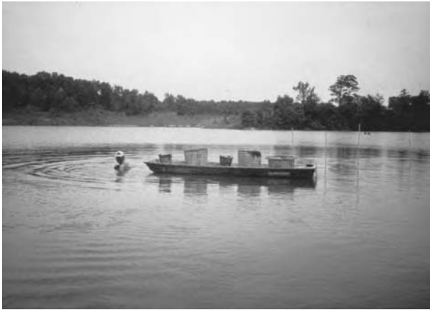
The muck barge in action. Muck from the pails is placed in tubs on the barge (flat-bottom boat). At the shore, the tubs are set on a two-wheeler and taken to a disposal area.
