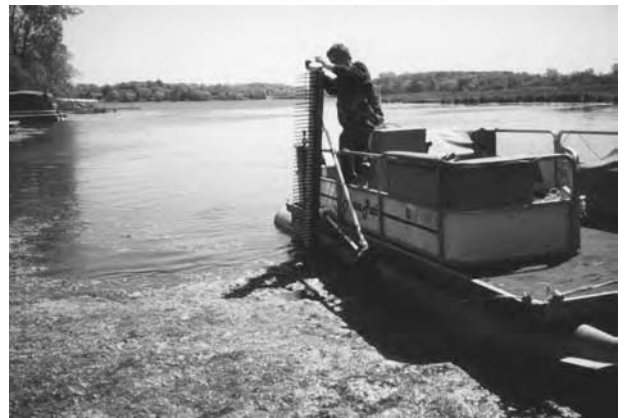
After the algae have been pushed to shore, the algae rake is lifted up and the pontoon goes out and makes another run. This system can also be used to gather floating aquatic plants that have been cut.
