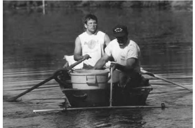
One person directs the boat, and another pumps the buffered alum into the water.
