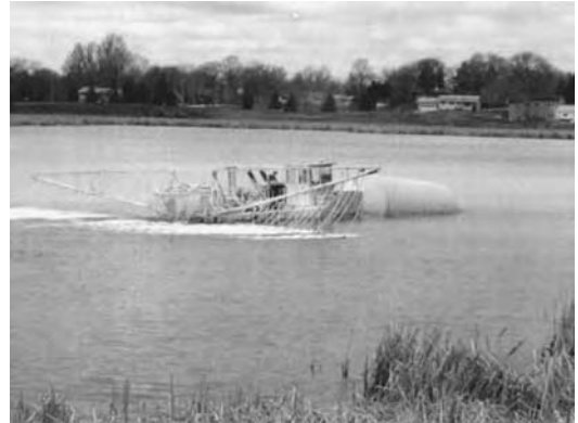
Calcium hydroxide applied to curlyleaf beds seems to reduce curlyleaf density in some cases. For this project, powdered calcium hydroxide was delivered from the floating tank, slurried, and applied to curlyleaf beds. This was a professional operation. On a smaller scale, you may be able to rig up your own slurry delivery system. Additional instructions are found in Serediak, M.S. et al., Lake and Reservoir Management, 18, 66-74, 2002. (From Sweetwater Technology.)
