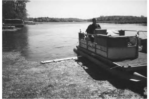
Other devices can be used to gather in filamentous algae as well. This is a weed rake (Beachcomber, discussed in Chapter 3) attached on a hinge to the pontoon and supported with floats in the water.
