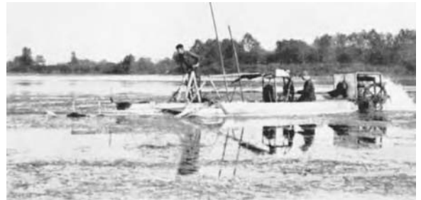
This cutter in the 1920s may be working on nuisance curlyleaf pondweed growth. (From Coates, P., Special Report on Lake Improvement , Ramsey County Engineering Department, St. Paul, MN, 1924.)
