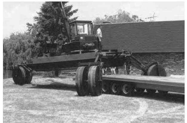
This is an amphibious backhoe. It can move from dry land to the water.
