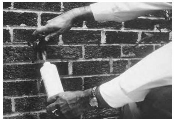
Testing well water can be done right from your tap. Make sure you run the water long enough to run out water that has been sitting in the tank. Do not touch the bottle opening. (From USEPA.)
