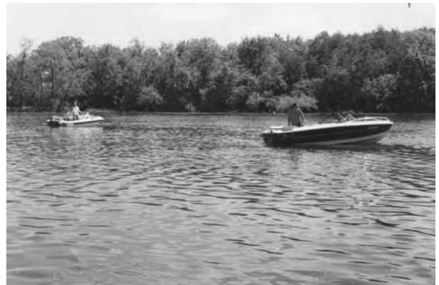
The boats start about 70 to 80 feet apart and then motor parallel through a weedbed. The weight of the weeds on the cable forces the boats to come together. This is a good time to stop. A minimum of 75-hp motors are needed, and there is some wear and tear on the lower unit.
