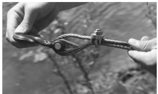
The cable is connected to a hook that attaches to the boats. To clean the weeds off the cable, one end is unhooked from the boat and the hook is removed. The boat with the attached end motors ahead and the cable slips out of the weeds wrapped around the cable.
