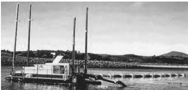
Dredge material has to be pumped to a disposal area. The pipes used for carrying material come in 15- to 20-foot sections and are coupled together. A float system is needed to keep them on top of the water.
