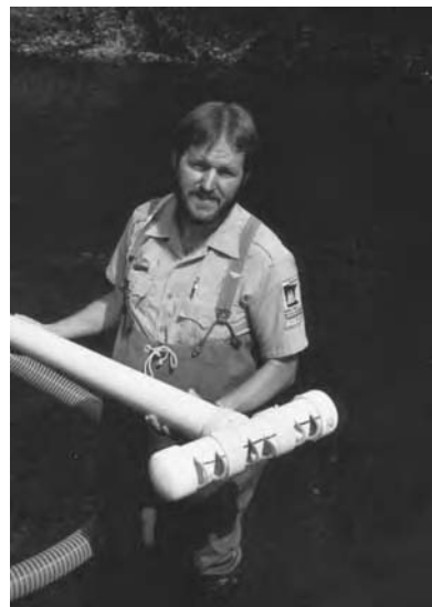
This intake was fashioned from a piece of PVC pipe 3 inches in diameter with 1-inch slits cut into the pipe.
