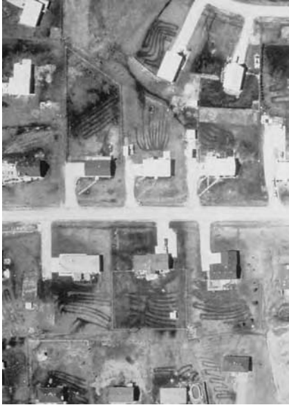
Color infrared photography can highlight drainfields with potential problems. (From USEPA.)
