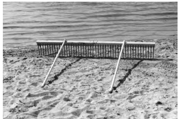
Two Beachcombers coupled together make a 6-foot-wide rake. A wooded dowel fits into the hollow tube of the rake head, and two rakes are held together. Attach a metal plate with bolts to complete the connection.
