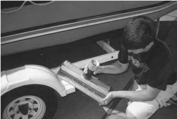
This intake was created using a swimming pool cleaning head and adding a sheet metal scoop.
