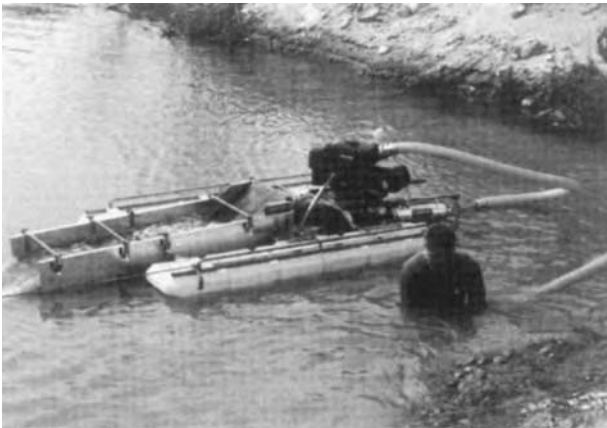
Conventional commercial gold dredges like this 5-inch dredge from Keene Engineering are effective at lifting sand, silt, and gravel. A drawback is that it cannot discharge material a great distance.
