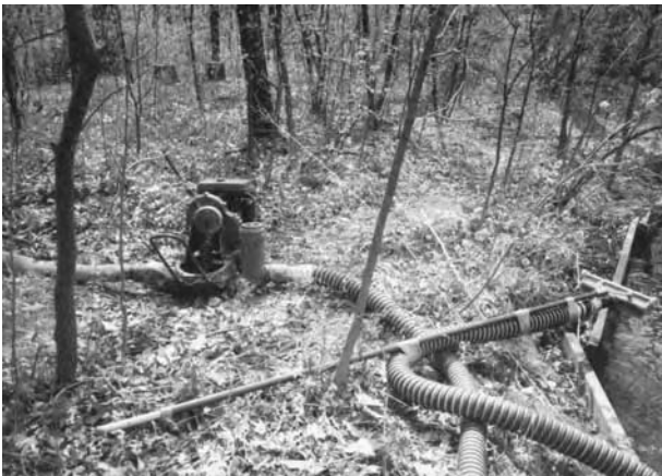
The diaphragm pump setup consists of an intake, suction hose, pump, discharge line, and the disposal area (not shown).
