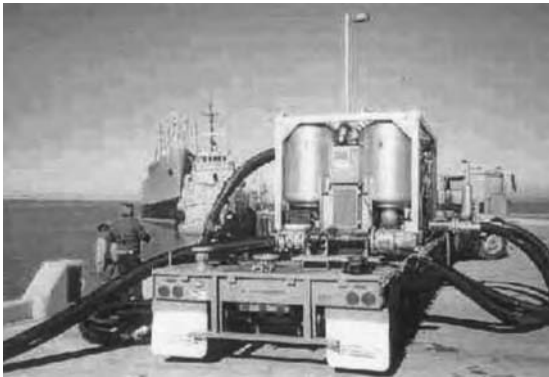
A CounterVac pump with a double-cylinder setup. Mounted on a trailer, the pump can be transported right to the edge of the pond or lake.
