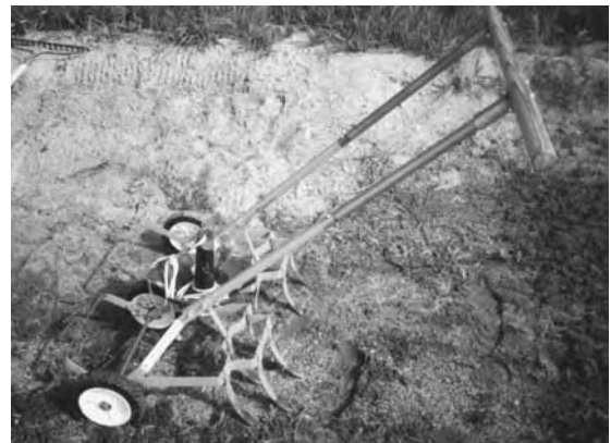
For lake work, it is more efficient to couple two cultivators together with a single axle. Three lawnmower wheels support the cultivator and make it easier to move around. The shovels have been reversed so the cultivator can be pulled rather than pushed in a lake. A single dowel at the top acts to connect the cultivators and serves as a pulling handle. It is easier to pull contraptions through plant beds rather than push them. Weight is added on the platform to promote better penetration by the shovels. The weight is a boat anchor.
