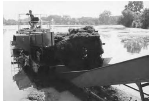
Harvester conveyor system transfers weeds to an on-land conveyor system and then to the back of a dump truck.
