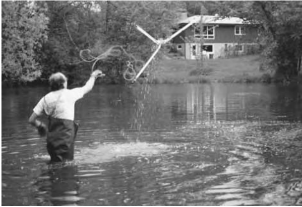
The hand-thrown, V-shaped cutter cuts a 3-foot-wide channel through weeds. One end of a rope is attached to the pole and the other end to your wrist. The cutter is thrown out and dragged back in.
