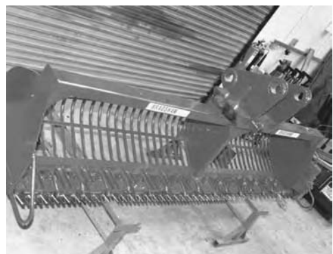
A twist on aquatic plant harvesters is this land-based harvester. The Bradshaw weed cutting bucket made in Peterborough, England, has a scissor-cutting action mounted at the bottom lip of the bucket. It is mounted on a long arm of a backhoe and is handy for cleaning canals and ditches from the bank.
