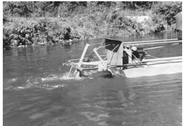
The paddle action propulsion on the Hockney underwater weed cutter allows it to travel through dense weeds without getting tangled.
