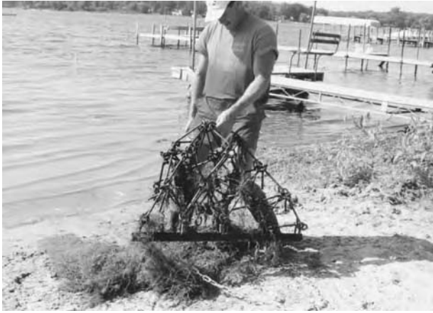
When the harrow is picked up in the middle, the biomass falls off.
