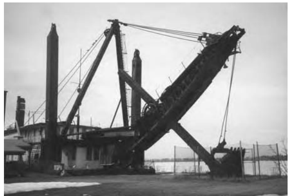
An 80-year-old, steam-driven dipper dredge in dry dock at a park in Wisconsin. Built by Bucyrus Co., Milwaukee, WI. The story is that the dredges were so well built that they never broke down and the Bucyrus Company went out of business.
