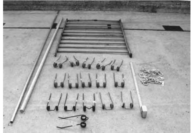
The basic components for building your own harrow include a frame, spring teeth, wooden dowels or conduit pipe, and U-bolts. In this case, the frame is a section of an iron railing.
