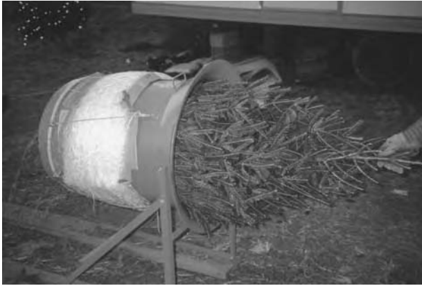
For projects that require a lot of barley straw, a Christmas tree bailer eases repackaging efforts. Christmas tree bailers cost about $350 and are available from O.H. Shelton and Sons (Coon Rapids, MN; Tel: 763-433-2854).
