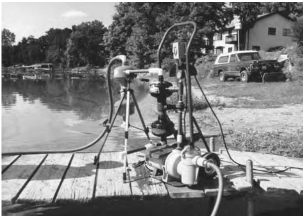
When two swirl units were put in series, algae removal efficiency increased.
