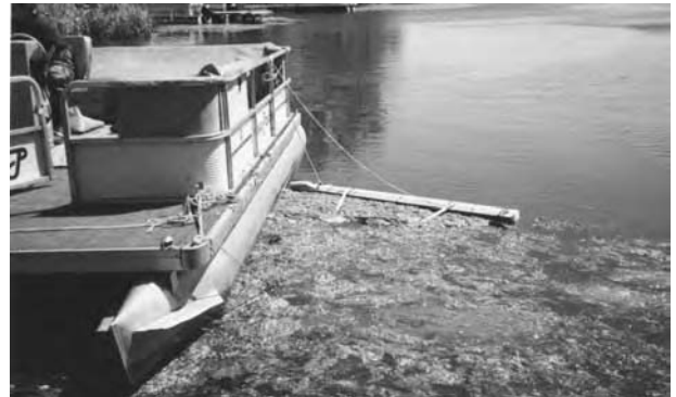
You can buy attachments from the Hockney Company to help push weeds to shore (mentioned later in the mechanical cutting section), or you can make your own weed-gathering devices. Several 3-foot wide rake sections were attached to a capped PVC pipe. The device is secured to a pontoon or boat. It is effective for pushing floating weeds to shore (as well as filamentous algae).
