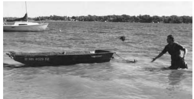
The weed barge can be just about any type of boat. The net is stretched over the length of the boat and plants are deposited on top of the net.
