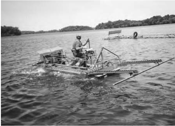
After a couple of years of pulling cutters, lake associations sometimes step up to a mechanical cutter like a Hockney weed cutter. It is more expensive but requires less labor and fewer volunteers. (From Virgil Leuhrs.)
