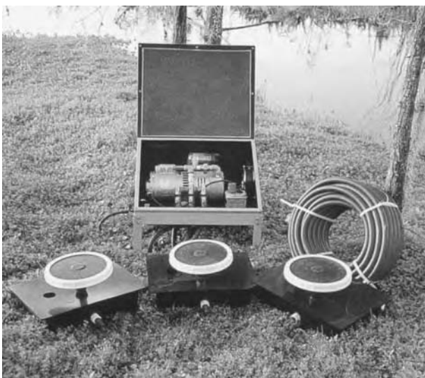
Components for conventional aeration include the air compressor (in a housing), aeration heads that convert the air to fine bubbles, and the air line. Electricity is needed to run the compressor. (From Vertex Water Features, Deerfield Beach, FL.)
