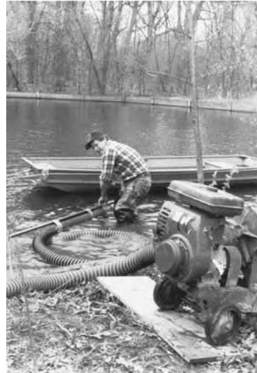
Diaphragm pumps are light and easily moved around the lake-shore. Their pumping capacity is less than the same-sized centrifugal pump but they pump a higher percentage of solids.
