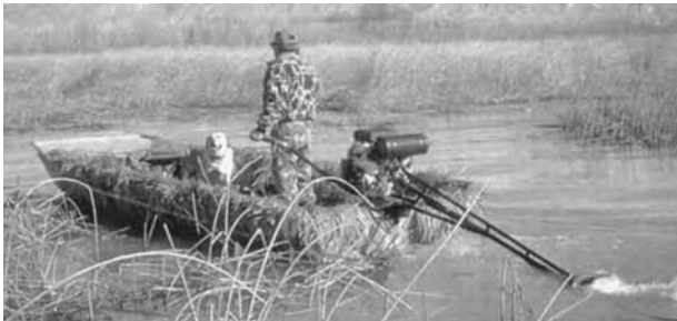
A 25-hp marsh motor supplements the reverse aeration mixing effort. You will have to design your own frame so you can work with the propeller through the ice.
