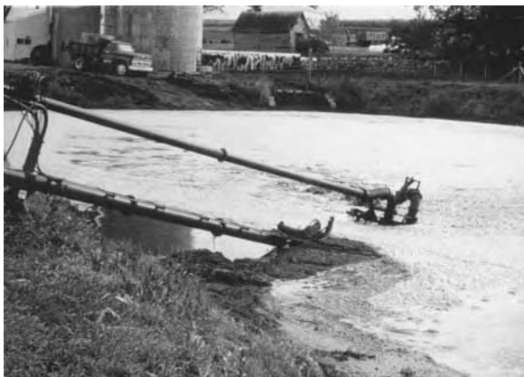
Crisafulli pumps come in a variety of designs for a variety of uses. They can work as a small-scale dredge but the intake is difficult to maneuver.
