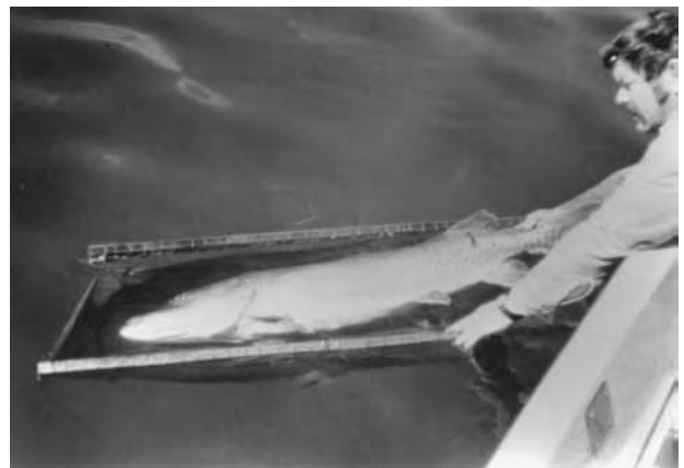
Fish cradles minimize fish handling and reduce stress to fish. (From Minnesota Department of Natural Resources.)
