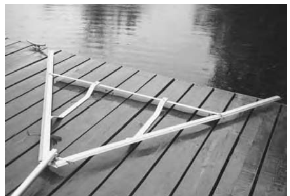
Both types of cutters—the 3-footer and 6-footer—will trim aquatic plants 2 to 4 inches from the lake bottom when pulled along at a slow speed with a jerking action. The 6-foot-wide boat-towed cutter rides on the skids along the lake bottom.
