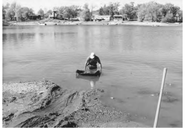
As the slusher is pulled in, push down on the handles when you have a full scoop. Once the lip is out of the sediments, you will not collect any more.
