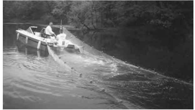
Drifting weeds in the middle of the lake are difficult to get to shore. The weed mass within the net generates severe drag and demands a lot of power to tow it to shore.
