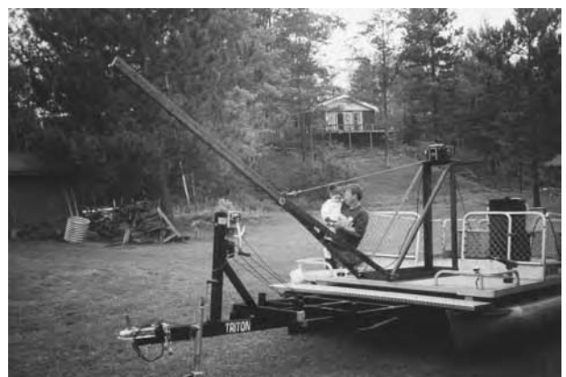
In fall, the barley bales were removed with a home-made lift constructed from an old pontoon boat and a hoist. The wet bales each weighed about 150 pounds. In many cases, the chicken wire had rusted out at the bottom.
