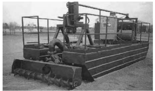
Here is a commercial dredge by LWT Inc. (Sommerset, WI). A hydraulic pump is the heart of the system. It can be remotely operated and runs off an electric motor. The horizontal auger suspends soft sediments that are sucked up by the intake in the center.
