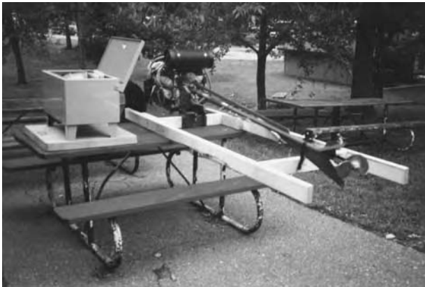
The basic equipment for reverse aeration is an air compressor (about \frac{1}{4} hp will work), air line, and diffuser head. A portable generator can supply power for the compressor. The duck boat motor or marsh motor can also be used to induce a low level of mixing under the ice.
