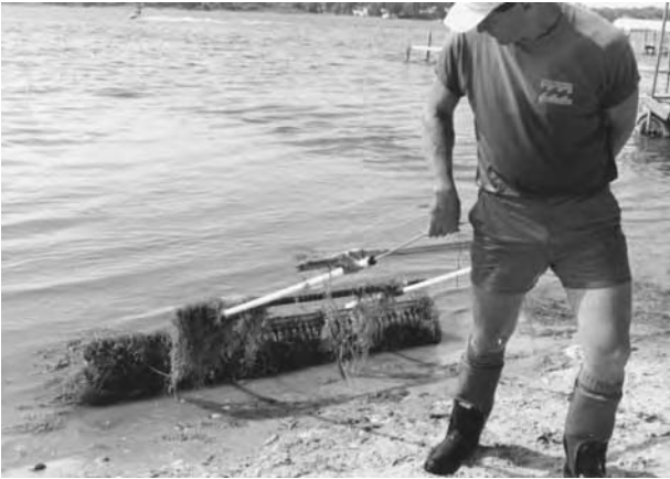
The Double Beachcomber is light and easily carried into and pulled out of the lake. Sometimes, adding extra weight at the rake head improves the bite into the sediments.
