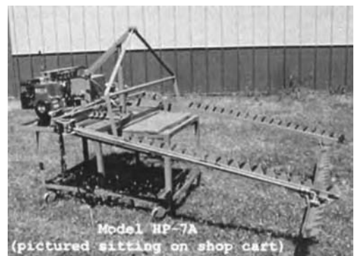
A slightly less expensive option is the hydraulically driven Hockney boat-mounted cutter. It cuts a 7-foot-wide path down to a depth of about 3.5 feet. The cutter is powered by a 5-hp Briggs and Stratton engine. It is mounted on boat length of at least 14-feet.
