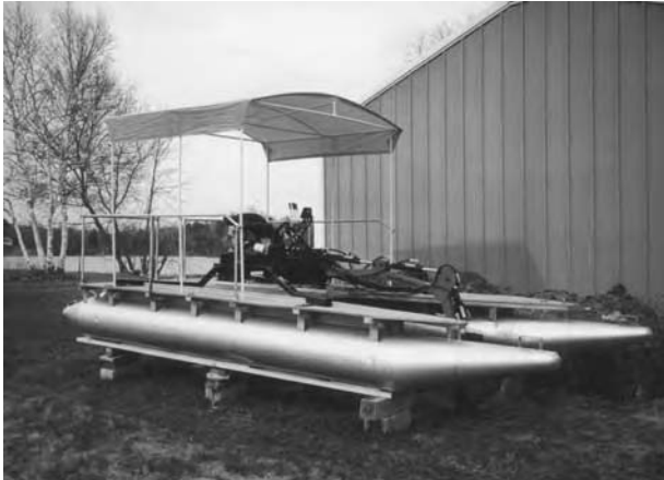
Mounting a backhoe on a pontoon takes some effort. The result is a device suitable for small jobs. The backhoe unit costs about $3500, and the pontoon costs range from $500 (used) to $4000 (new).
