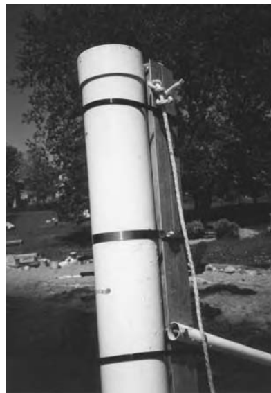
The float system on the rake is a 4-inch capped PVC pipe attached with hose clamps.
