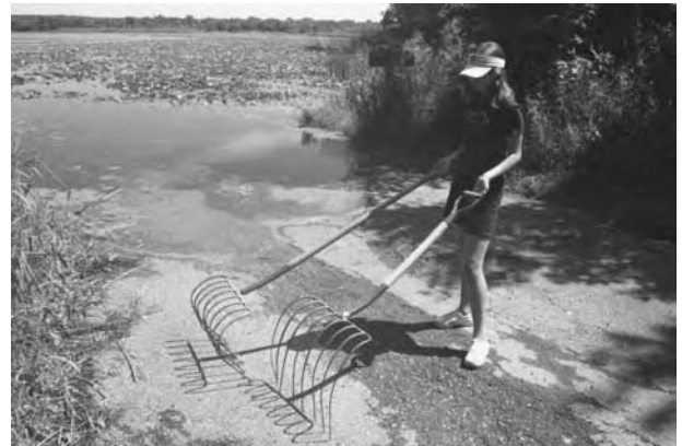
The silage fork rake is modified from a silage fork. When raking an area, it accommodates bushy weeds but will miss stringy weeds because the tines are about 2.5 inches apart.
