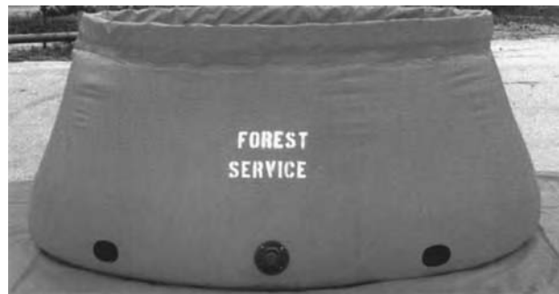
Portable water tank is self-supporting and can be set up by one person. Sizes range from 500 gallons ($650) to 5000 gallons ($3000).
