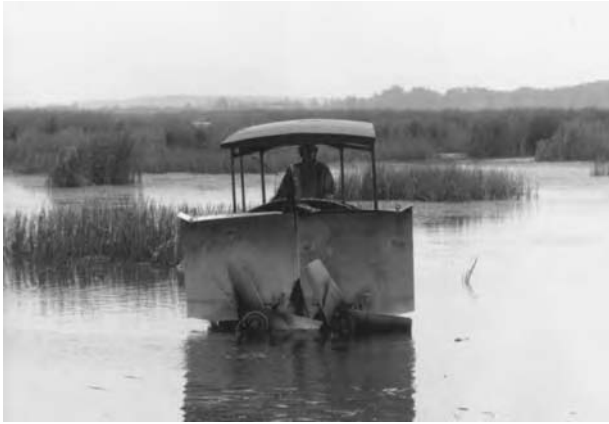
A cookie cutter represents a heavy-duty way to cut channels through cattail mats. This is an older model used for wetland management at the Carlos Avery Game Refuge in Minnesota.
