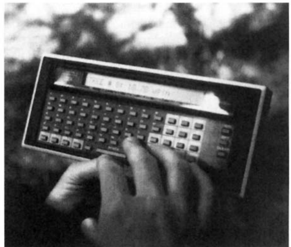
Figure 11.19 Sample tree measurements are entered directly into this small, battery-operated computer, which is taken into the forest. The computer is capable of performing all the statistical calculations necessary to prepare a stand and stock table (Table 11.5).
