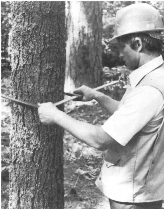
Figure 11.7 Forester using a caliper to measure a tree diameter at breast height (dbh).
