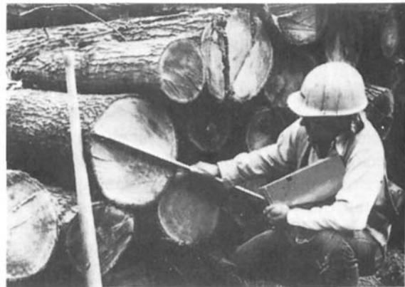
Figure 11.1 First step in scaling: determining the diameter inside the bark on the small end of the log.
