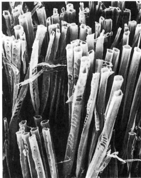
Figure 20.15 Scanning electron micrograph of a cluster of eastern white pine elements after pulping or maceration of a small wood cube. (Courtesy of Wilfred Cote and Syracuse University Press.)
