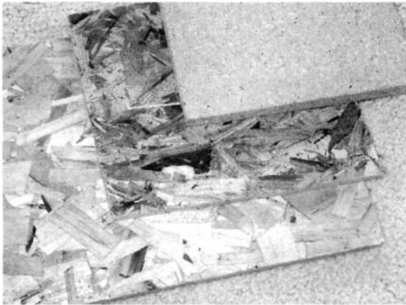
Figure 20.10 Manufactured wood products include flakeboard (at top of stack), OSB (at middle of stack), and particleboard (at bottom of stack).
