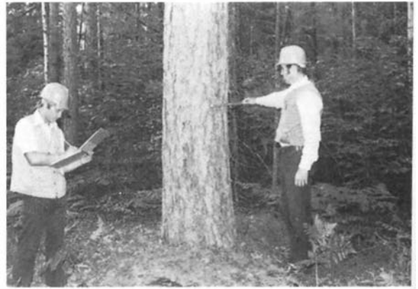
Figure 11.8 Field crew in the process of observing and recording species and tree diameters on a plot. Diameters are being measured with a Biltmore stick held at a fixed distance from the eye. Observations with this instrument are based on the geometric principle of similar triangles.
