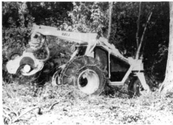
Figure 19.1 Rubber-tired feller-bunchers are productive—this highly maneuverable three-wheeled model is well-suited for thinning.
