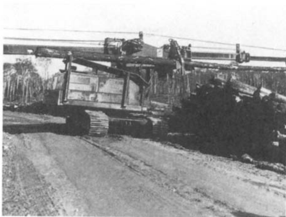
Figure 19.4 A stroke delimiting machine is a safe and effective mechanical delimiting machine for most softwood species.
