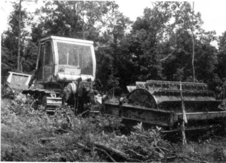
Figure 13.7 Mechanical site preparation reduces competition from advance regeneration and shrubs, and provides a more favorable seedbed for establishment of preferred species. The rolling brush cutter shown here can achieve these results without scraping away or displacing topsoil and nutrients.
