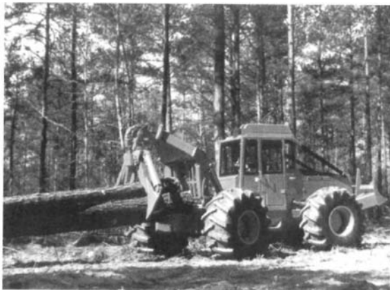
Figure 19.5 A rubber-tired grapple skidder, combined with a feller-buncher, forms a productive and cost-efficient logging system.
