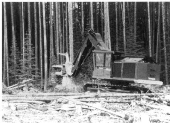
Figure 19.2 This track-mounted feller-buncher generates low ground pressure and minimizes soil compaction and rutting.
