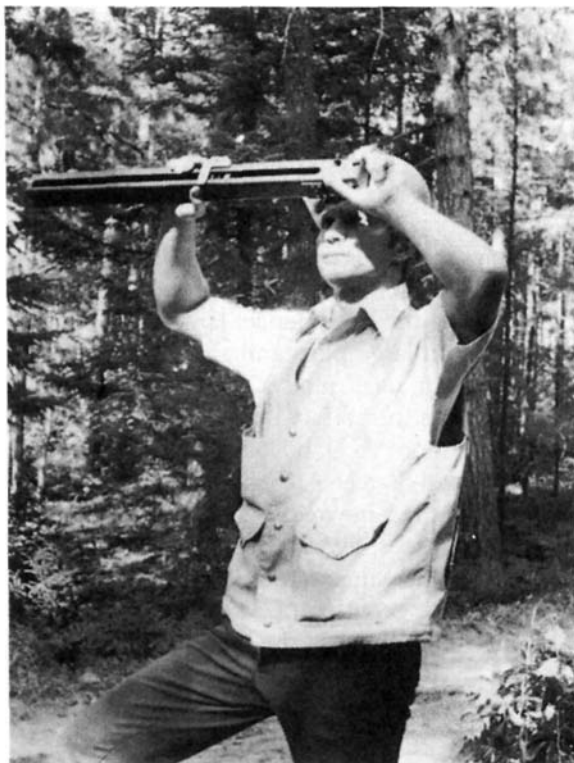
Figure 11.12 Observation of the upper-stem diameter with a Wheeler optical caliper.
