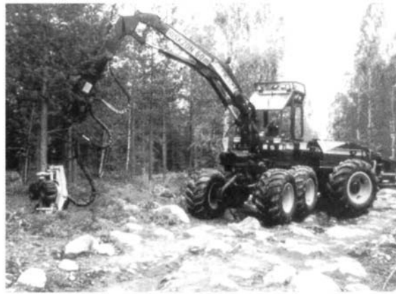
Figure 19.3 A harvester is a multifunction machine that fells, delimits, tops, measures, and bucks the tree at the stump.
