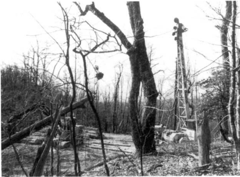
Figure 19.7 A skyline cable yarder system can harvest timber on steep mountain slopes with minimum soil disturbance.
