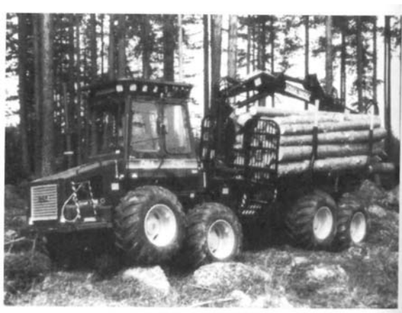
Figure 19.6 A forwarder loads and transports cut-to-length logs from the stump to a roadside landing.
