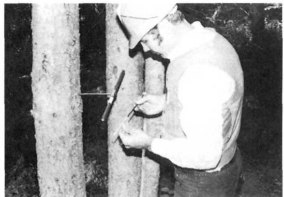
Figure 11.13 Tree age determination with an increment borer.
