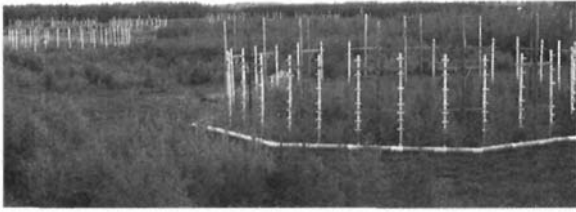
Figure 4.16 In an effort to generate accurate predictions of forest response to atmospheric CO 2 enrichment, scientists have constructed three FACE (free-air CO 2 enrichment) facilities in the eastern U.S. Each facility consists of several large rings of vertical pipes surrounding stands of trees. Based on measures of meteorology and atmospheric chemistry inside the ring, CO 2 is released from vents in a subset of the pipes. Using this approach, stands of trees can be continuously exposed to a target CO 2 concentration with otherwise minimal perturbation of their environment. The rings shown here enclose stands of trembling aspen ( Populus tremuloides ), white birch ( Betula papyrifera ) and sugar maple ( Acer saccharum ) at a facility in northern Wisconsin. (Photograph by Evan McDonald.)
