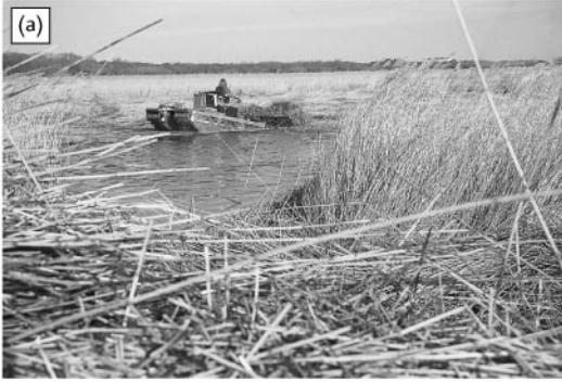
Fig. 8.16 Mechanised cutting and removal of common reed. Where small-scale mowing of fens for thatch and litter is no longer economic, larger-scale machines can be used to cut and remove vegetation to retard succession.
