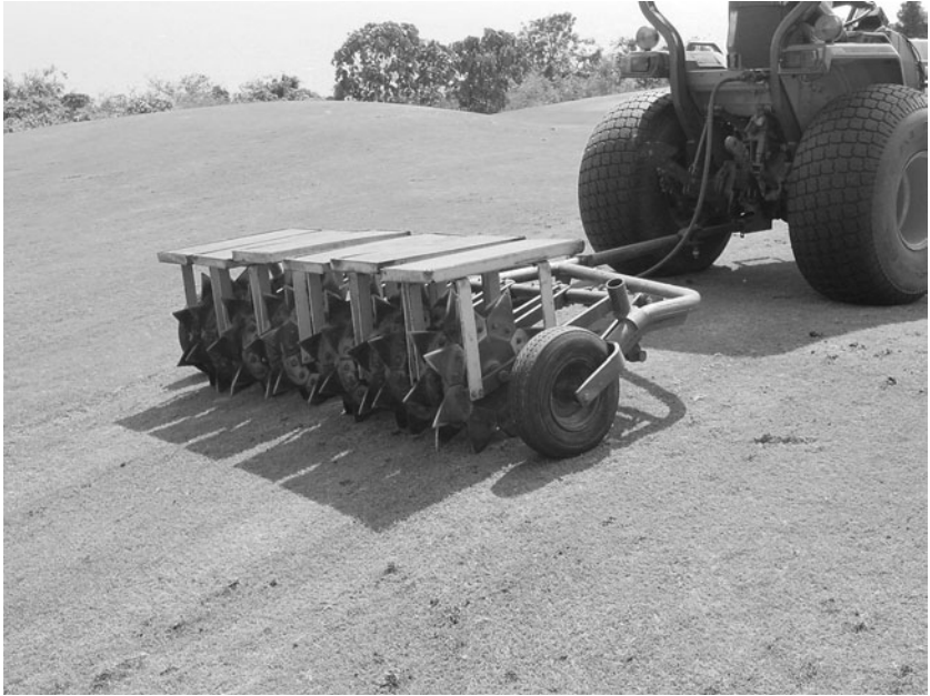
Fig. 8.4. Rotating flat tines slice vertically through the turf and soil, reducing compaction and improving aeration.
