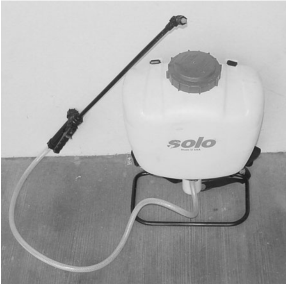
Fig. 11.5. Hand sprayers are used on small or hard-to-reach areas and usually have only one nozzle.
