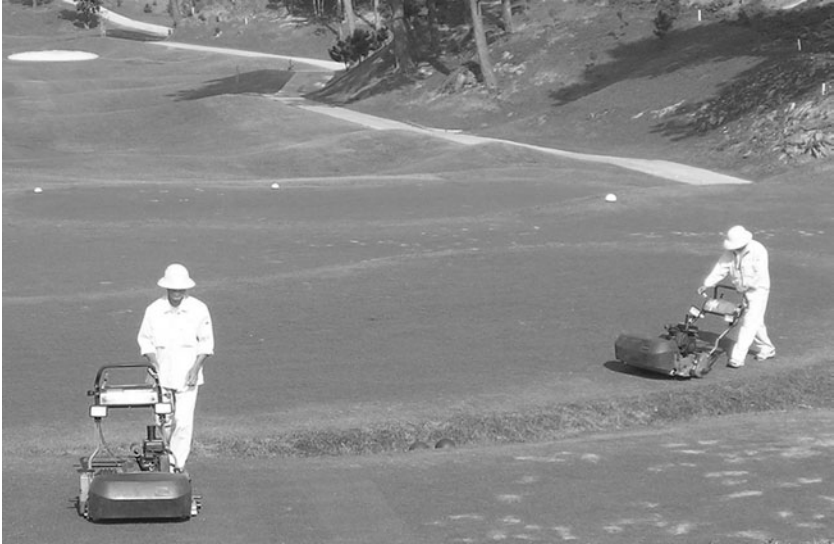
Fig. 9.3. For mowing of putting greens and tees, walking mowers are preferred. They provide the most accurate cut and minimize the chances of accidental scalping.
