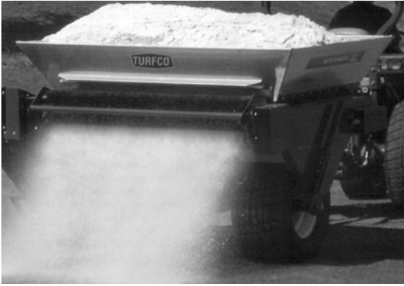
Fig. 8.7. Top-dressing, the application of a thin layer of soil over a turf-grass area, is usually used to cover thatch or to smooth the playing surface.
