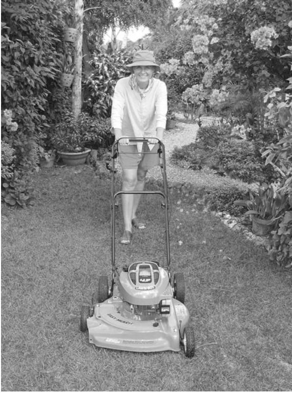
Fig. 6.7. The blade of a rotary mower spins in a horizontal plane, striking and severing vertically growing leaf blades.
