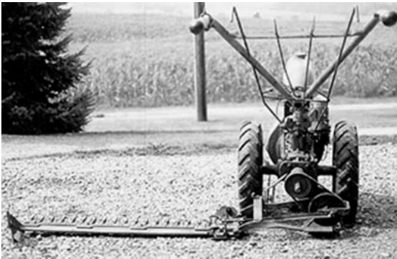
Fig. 6.9. A sickle-bar mower, used for cutting long grass and tall weeds on low-maintenance turfs.
