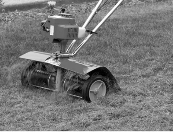
Fig. 8.6. The blades of the vertical mower cut vertically into the turf canopy, severing lateral stems and removing thatch that develops on the surface.
