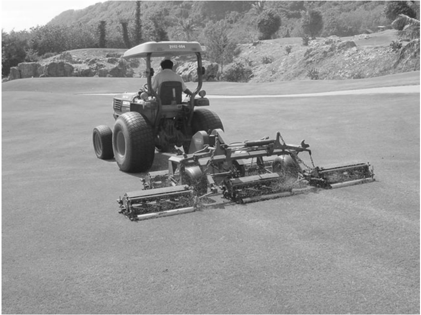
Fig. 9.9. Reel-type gang mowers pulled behind a tractor are one of the most popular types of mowers used on golf course fairways.
