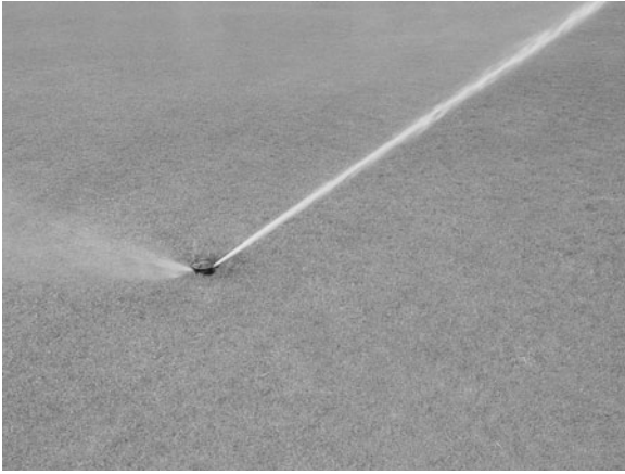
Fig. 7.5. Rotary sprinkler shooting two different streams of water spray.
