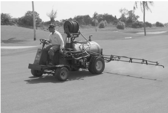
Fig. 11.3. Boom-type sprayers assure the most uniform distribution of pesticide over the turf area.
